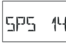
Speed stage only displayed if speed control is activated (ESR21-D only)
