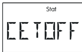
Collector - excess temperature - cut-off is active
