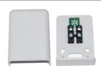
AUSPT – air temperature sensor with integral surge protection, can be used as an outside temperature sensor for heating system controllers, PT1000 characteristics, Permissible temperature range: -30 °C to +50 °C Dimensions (W x H x D): 40 x 54 x 23 mm
