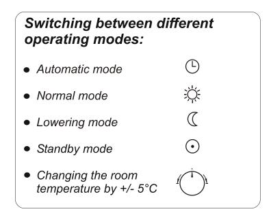
The room sensor is used as a command and temperature measurement instrument for the Technische Alternative controllers. The reported signal corresponds to the room temperature changed using the rotary knob. The following signals are forwarded to the controller according to the switch setting:
