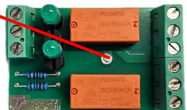
The auxiliary relay can be connected across any two analogue outputs if these are programmed as **switching outputs**.
