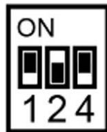
Position of DIP switches acc. to example.
