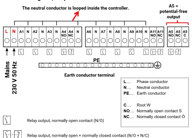
For maximum current load of the outputs, see the **technical data**.
