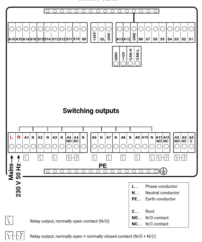
Caution: Output A5 is potential-free, i.e. is not connected to the mains power.
