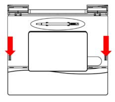
3. After removing the controller, unhook the closures (arrows in the diagram on the left) by pushing them down (using a small screwdriver or the programming stylus) and remove the mounting base cover from the lower section.
