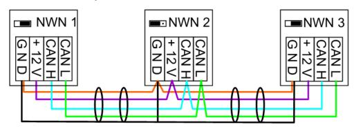
Each CAN network is to be provided with a 120 ohm BUS terminator at the first and last network subscriber (= termination). This is achieved with a plug-in jumper at the back of the controller. Each CAN network therefore always has two terminators (one at each end). Branch cables or a star topology are not permissible for CAN wiring.
