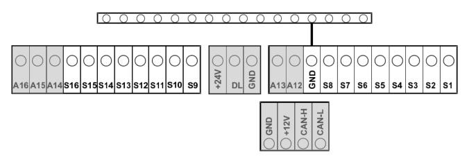
Sensors are always connected across the relevant sensor terminal (S1 – S16) and sensor earth (GND). An earth strip is located at the top of the mounting base. A connection is established from this strip to the GND terminal.
