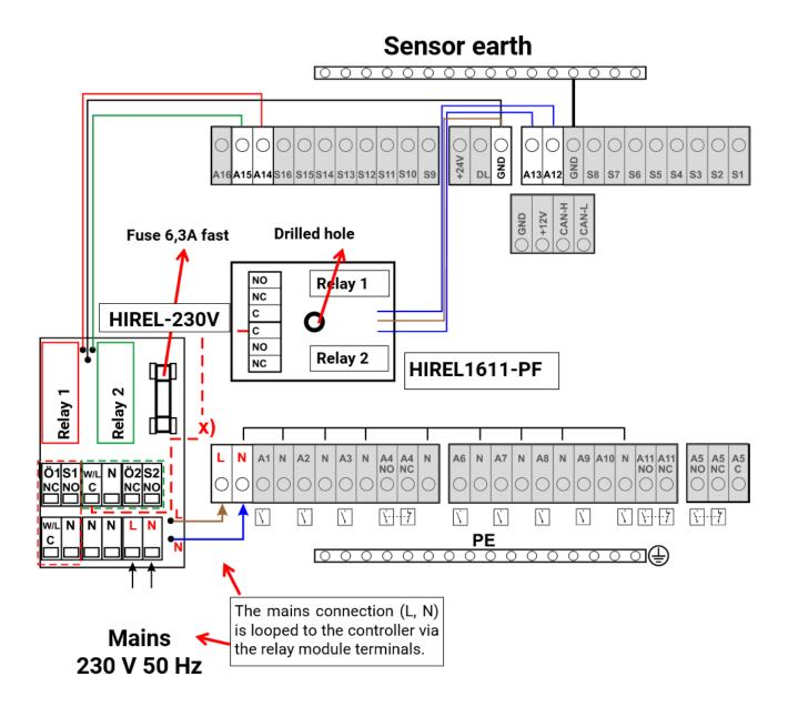
**X)** This connection enables the HIREL-PF relay contacts to switch the phase conductor (230 V) to become conductive. As a consequence the relay outputs are no longer potential-free. They are secured with the fuse of HIREL-230V.
