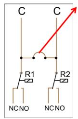
**Drilled hole**: The relay contacts are - without connection x) - potential-free, for which both roots (C) have been connected at the factory.
