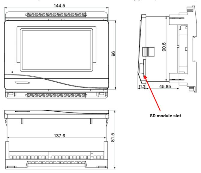
**Cut-out dimensions** for controller **UVR16x2S**: 138 x 91 mm, installed depth including terminal mounting plate: 70 mm
