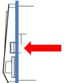
The two lateral locking clamps also enable the controller to be clicked into a **sheet steel front plate**.
