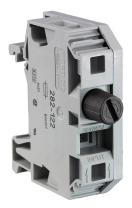
The SKL5x20 fuse terminal (including 6.3 A fast acting fuse) is used for external protection of the UVR610 controller. The internal fuse of the UVR610 can only be replaced at the manufacturer's factory. By connecting the fuse terminal to L1, the internal fuse of the device is bypassed. The fuse in the fuse terminal can be easily replaced on site.
