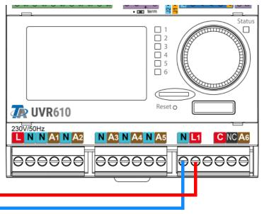
The fuse terminal is connected to 11. The direction as shown in the connection diagram must be observed (see "INPUT" printed on the top).
