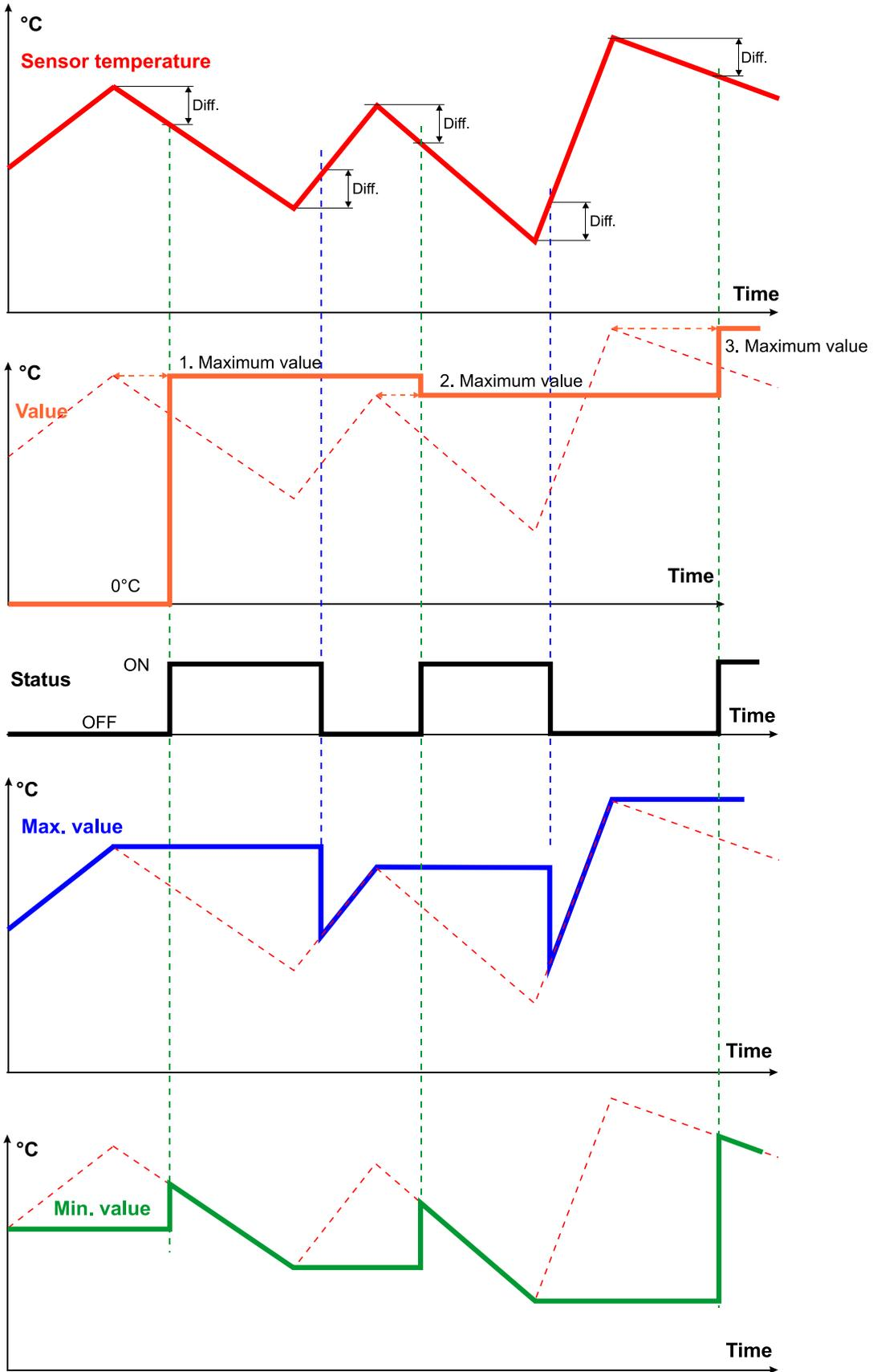
Graph for slope detection / positive slope / no reset signal / quasi peak
