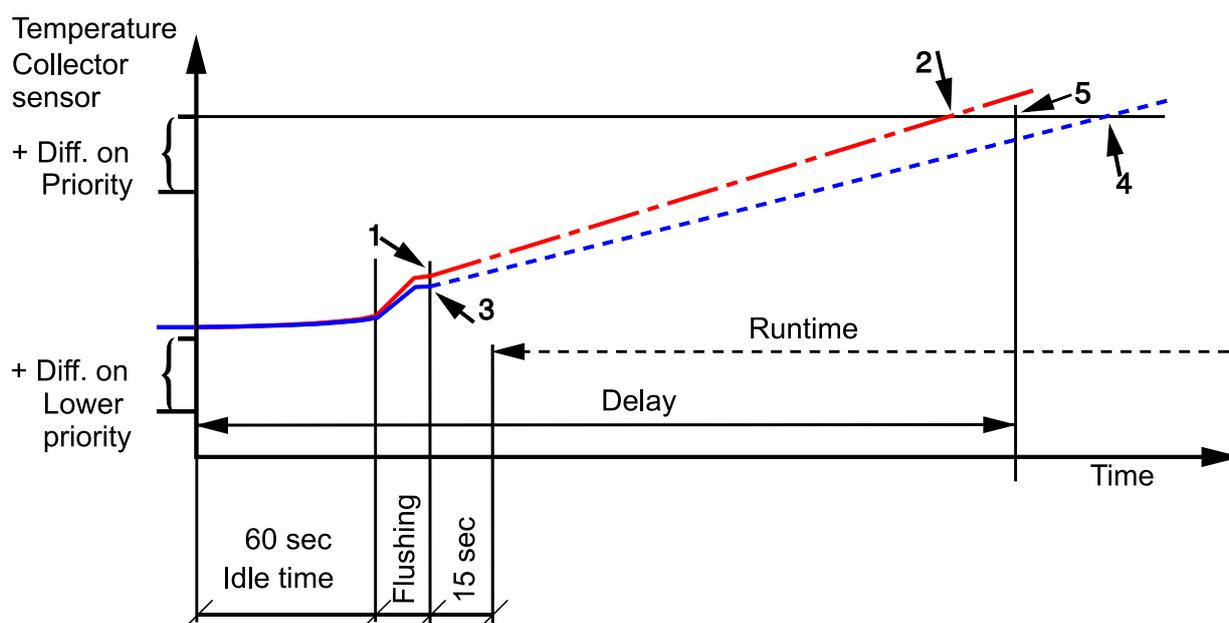
The device monitors the collector temperature while the lower priority consumer is being charged. If, while the pump is running, the collector temperature once again reaches the **start** differential (collector – reference) for the consumer **currently** being charged, the priority timer will be activated. If a radiation sensor is being used, the radiation level must exceed a threshold value, instead of the temperature differential.
