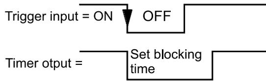
**Retrigger = Yes:** If the trigger input is switched ON within the blocking time, the blocking time will restart if the trigger input is switched back OFF **within the original blocking time**.
