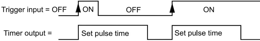
The trigger slope is **positive** if the input status changes from OFF to ON or from switch open to switch closed (= closing). This is shown in the example above.
