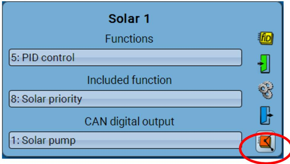
**Functions:** An output variable from **Solar** is linked to an input variable of the **PID control** function.
