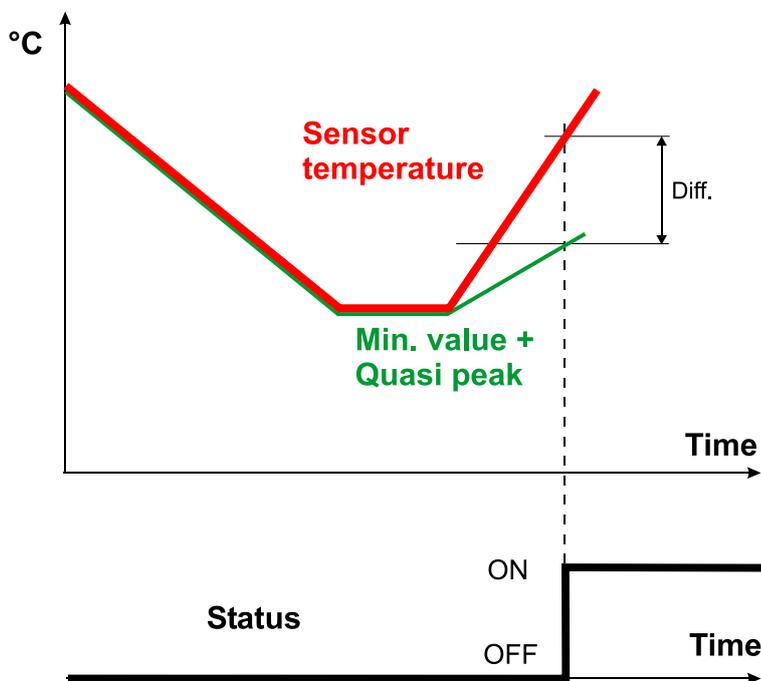
Graph for slope detection / negative slope / no reset signal / quasi peak
