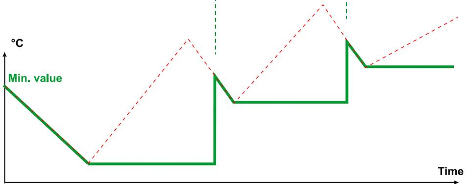
Graph for slope detection / positive slope / reset signal / no quasi peak
