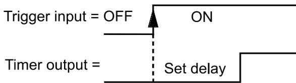
**Minimum runtime:** The ON signal at the trigger input switches the output on immediately. If the input drops during the minimum runtime (OFF), the output remains switched on anyway until the minimum runtime has elapsed. The output will remain switched on if the trigger input is in status ON when the minimum runtime has elapsed.
