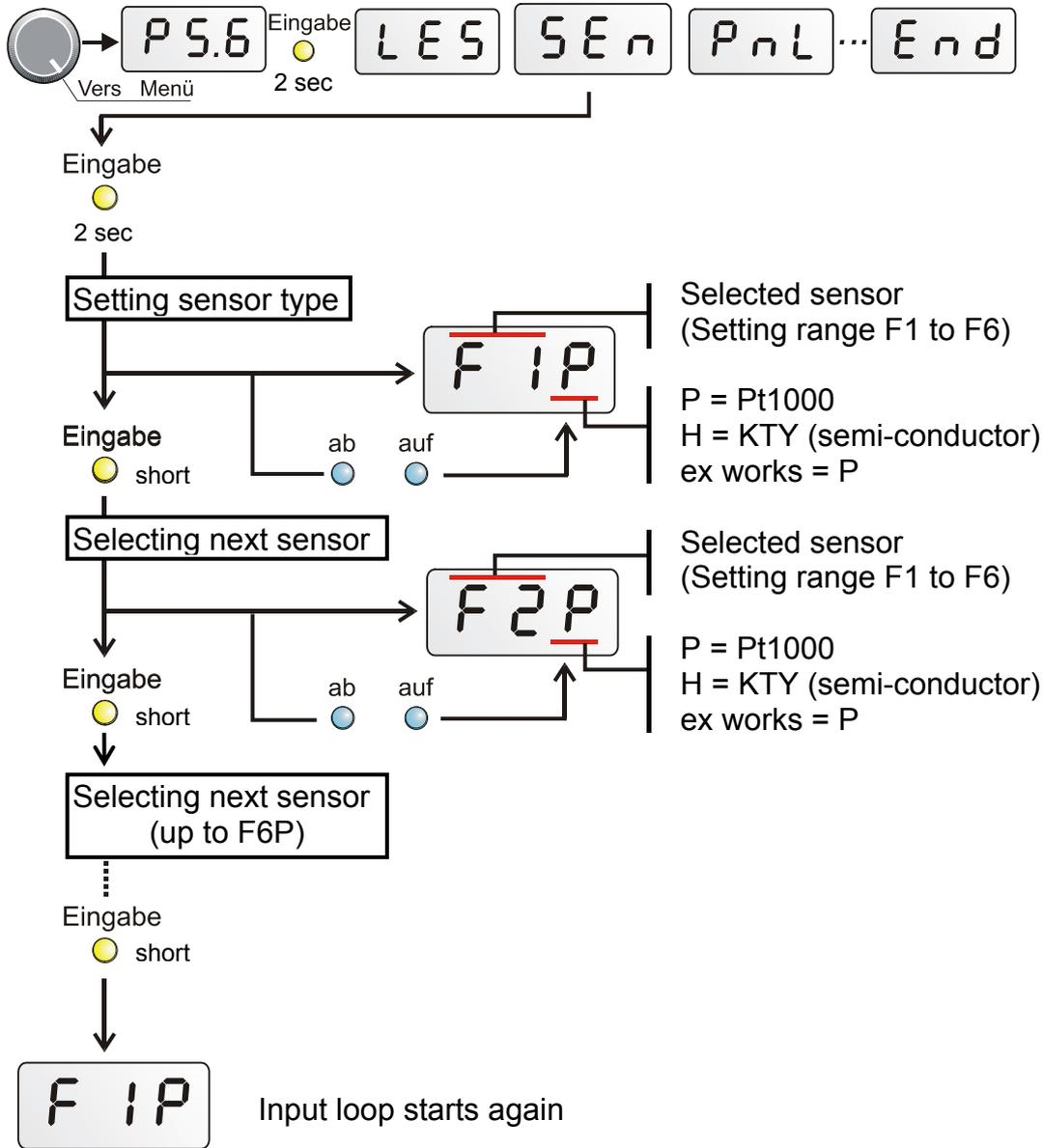
Exit from menu happens by pressing the yellow „**Eingabe**“ key for 2 seconds, turning the selector switch or automatically after one minute.
