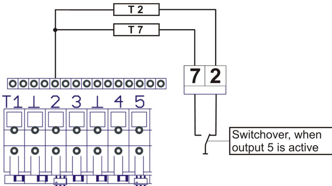
The temperature of sensor **T7** is displayed instead of sensor **T2** when output **A5** is active.
