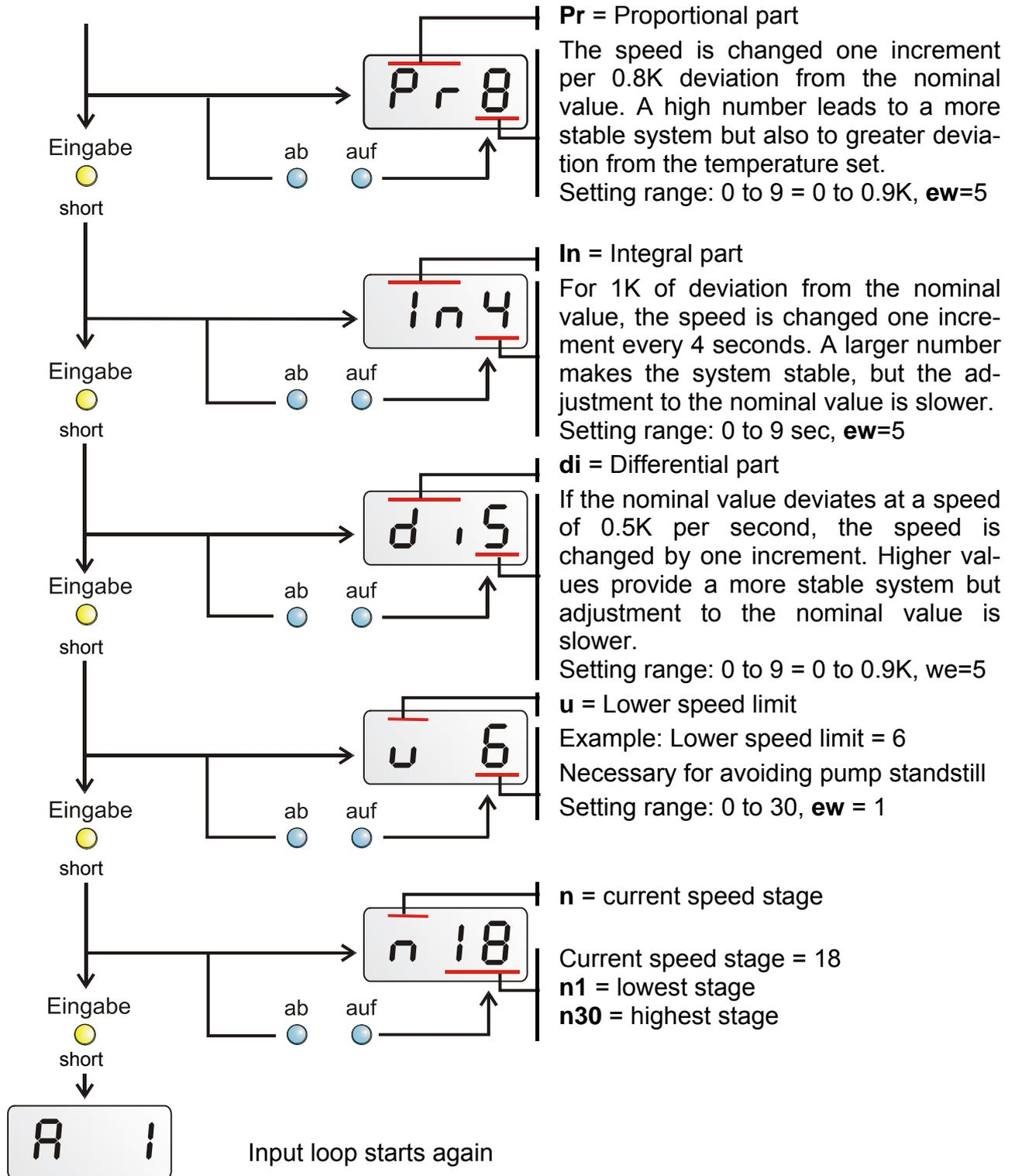
Exit from menu happens by pressing the yellow „Eingabe“ key for 2 seconds, turning the selector switch or automatically after one minute.
