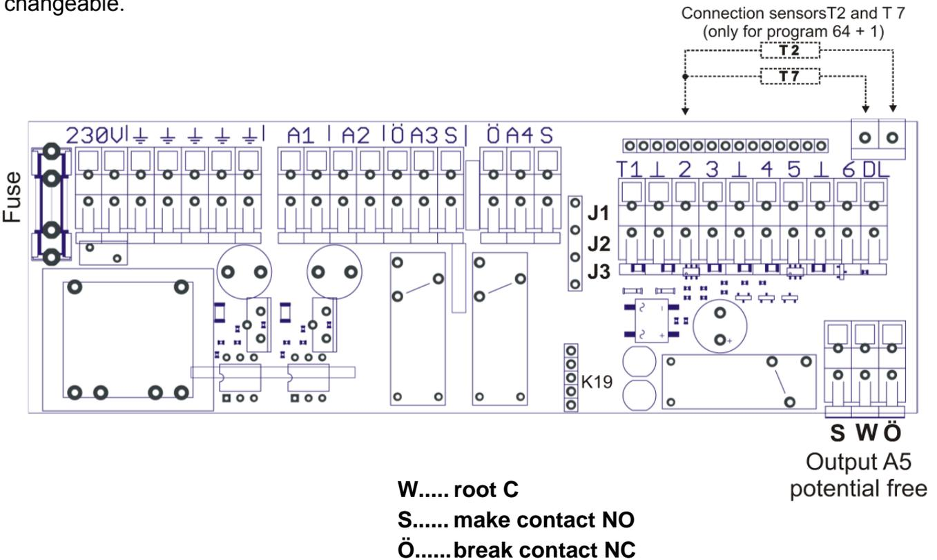
The relay output A4 can be made potential-free by setting the **jumpers** J1-J2-J3. For this purpose the jumper J2 must be set in the center instead of jumpers J1 and J3 (standard).
