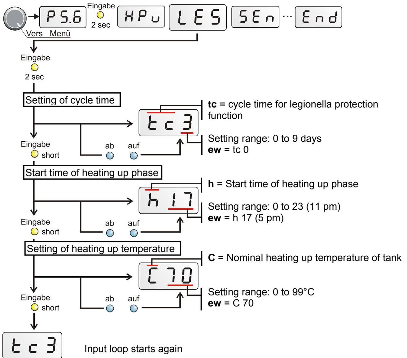
Exit from menu happens by pressing the yellow „**Eingabe**“ key for 2 seconds, turning the selector switch or automatically after one minute.
