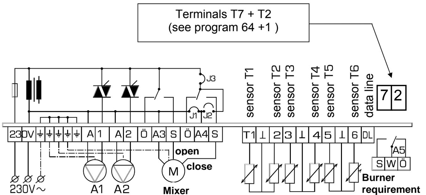
The fifth output **A5** is in the area of sensor terminals, which has a potential free switch-over contact. The connections W (root C) and S (make contact NO) are normally used for burner requirement.
