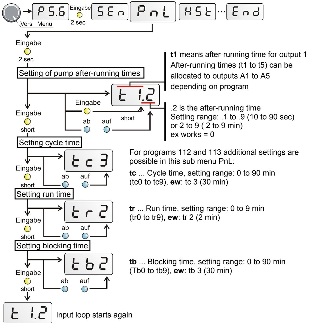
Exit from menu happens by pressing the yellow „**Eingabe**“ key for 2 seconds, turning the selector switch or automatically after one minute.
