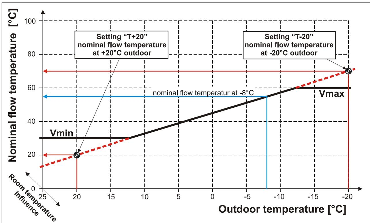
Looking at the diagram it is possible to detect the nominal flow temperature at a certain outdoor temperature.
