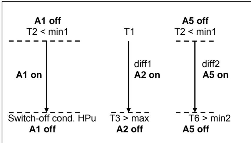
**Program 83:** **A5** is a hot water tank feed pump. Therefore the sensor **T6** is situated in the boiler. **Note:** **T6** must be set as standard sensor (**Std**) (see selector switch position **Mod – Par**).
