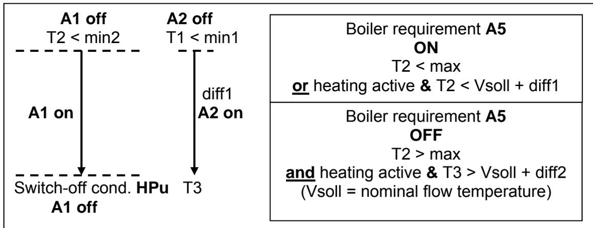
**Program 36:** Heating circuit pump and burner requirement are separated.
