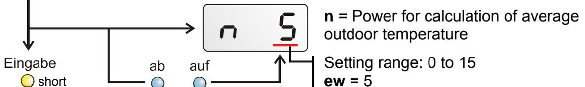
**i** The controller calculates the average value of outdoor temperature during integration time of  $2^n$  minutes.  $N = 5$  means, that the average value is calculated over  $2^5 = 32$  minutes.
