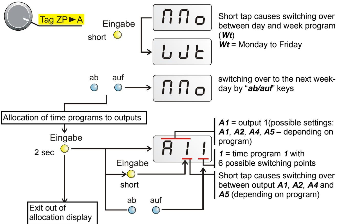
Exit from menu happens by pressing the yellow „**Eingabe**“ key for 2 seconds, turning the selector switch or automatically after one minute.
