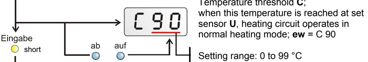
**Mixer behavior when heating circuit pump is switched off**
