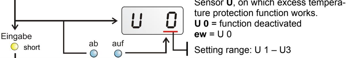
**Temperature threshold for excess temperature protection function**
