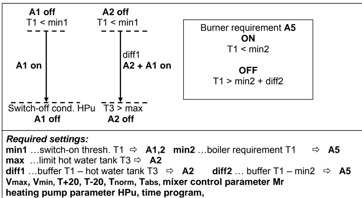
**A1 = T1 > min1 & (heating = active) or A2 (hot water requirement)**
