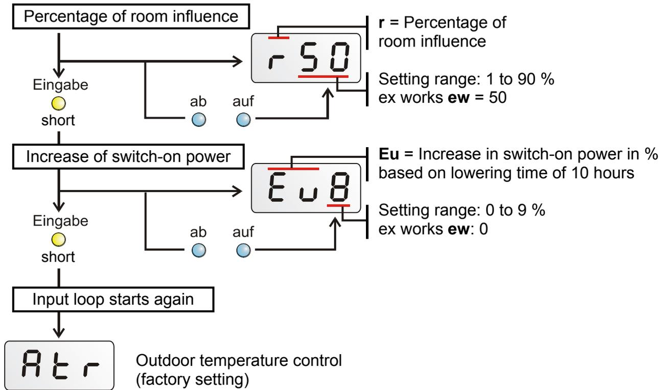
Exit from menu happens by pressing the yellow „**Eingabe**“ key for 2 seconds, turning the selector switch or automatically after one minute.
