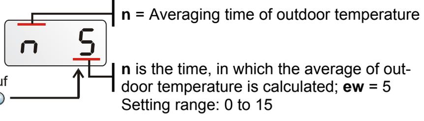
**i** The controller calculates the averaging time of outdoor temperature over an integration time of  $2^n$  minutes,  $n=6$  means an average time of  $2^6 = 64$  minutes.
