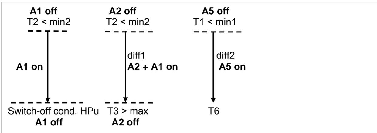
$$A1 = T2 > \text{min}2 \ \& \ (\text{heating} = \text{active}) \ \text{or} \ A2$$
