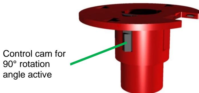
If the control cam has been broken out, but is no longer required, then it can be twisted by 180° and inserted into the groove, so that it can no longer actuate the limit switch:
