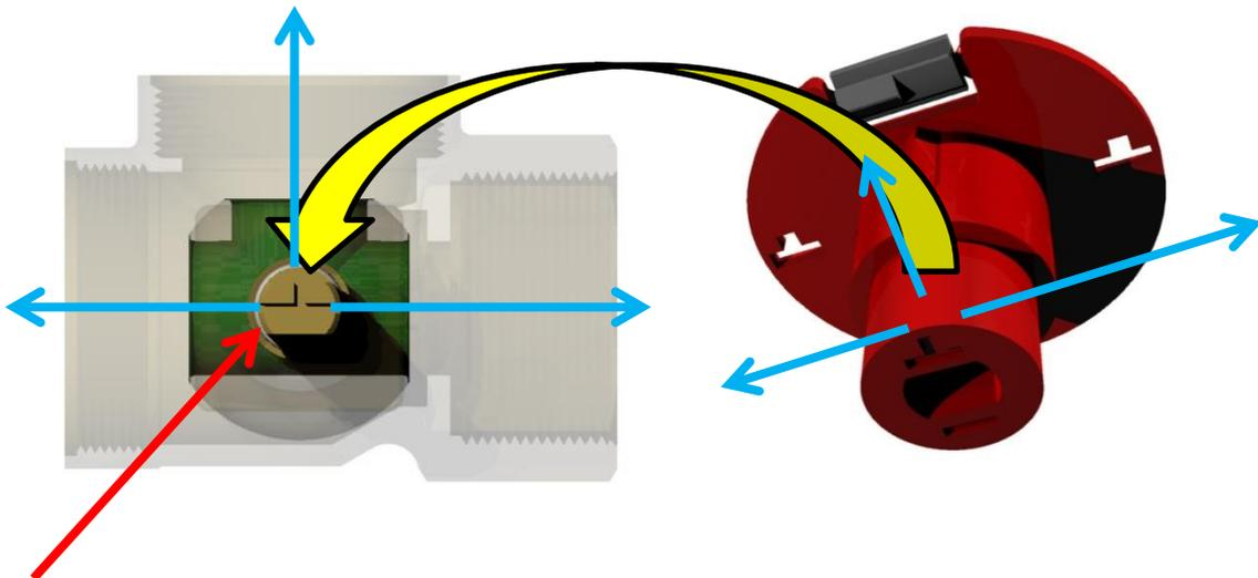
The **marking** on the valve shaft indicates the position of the ball valve.
