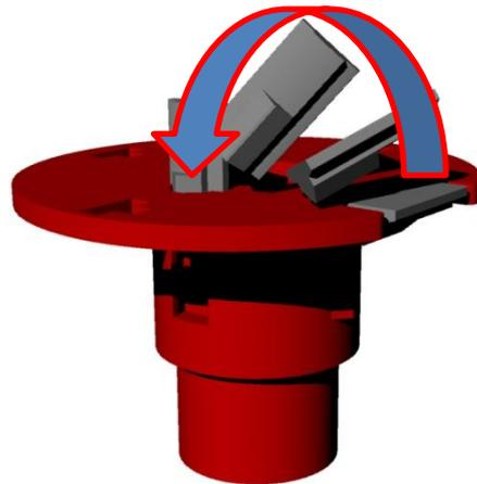
View of the correctly inserted 90° control cam
