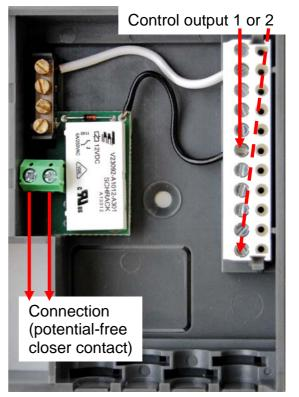
The relay module is connected to the sensor earth and a control output in accordance with the above images. The 4-pole earth strip is enclosed for the ESR31 controller.
