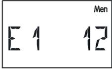
**Example:** The external sensor 1 has address 1, the measured room temperature is imported without offset values (index 2). In the controllers ESR31, UVR61-3, UVR63 and UVR63H (version 5.0 up to 7.1) only the measured room temperature can be evaluated without offset values (index 2); the sliding switch and the rotary knob have no purpose with these controllers. This value can subsequently be allocated to a sensor value (menu ENTER/Men – SENSOR).
