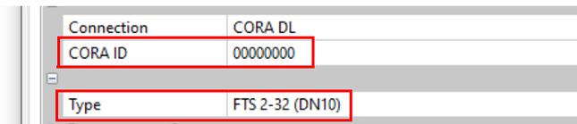
A double click leads to the parameters of the device. The type and CORA-ID are entered here.
