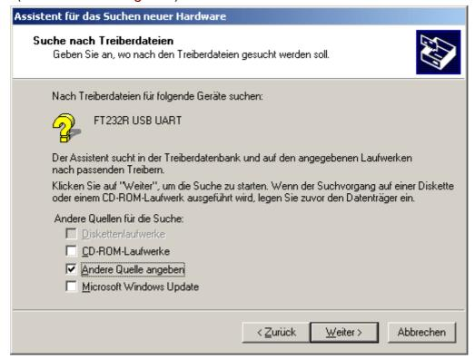
**4.** In the next step the path to the driver files must be specified: Windows 2000: <...\USB-Treiber\Win2kXp>
