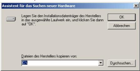
**5.** Click "Browse" ("Durchsuchen") to select the appropriate path and the .INF-file required for the installation. For the USB controller installation, <**USB Serial Converter>**, the file "**ftdibus.inf**" must be selected.
