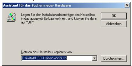
**12.** Click "Browse" ("Durchsuchen") to select the appropriate path and the .INF-file required for the installation. For installation of the virtual COM port, <**USB Serial Port**>, the file "**ftdiport.inf**" must be selected!
