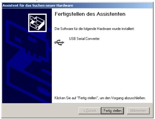
**6.** The hardware wizard continues with installation of the driver for the virtual COM-port (*USB Serial Port*). This driver is installed using the same procedure as the previous driver.
