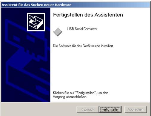
**8.** The hardware wizard continues with installation of the driver for the virtual COM-port (*USB Serial Port*). This driver is installed using the same procedure as the previous driver.
