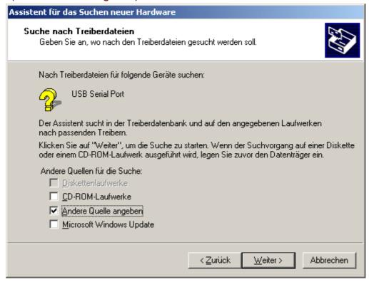
**11.** In the next step the path to the driver files must be specified: Windows 2000: <...\USB-Treiber\Win2kXp>
