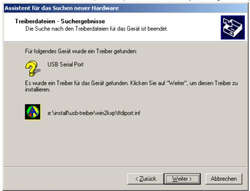
**14.** After successful installation of the driver for the virtual COM port (*USB Serial Port*), installation of all the components necessary for communication via the USB interface is completed by clicking "Finish" ("Fertig stellen").
