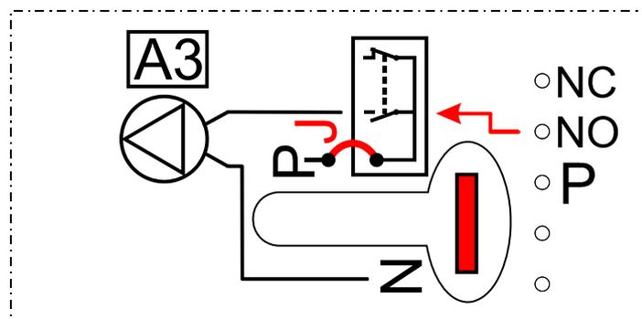
With the jumper **J** in place, output 3 is **not** potential-free.
