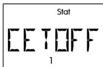
Collector – over temperature switch-off active (no error occurred)
