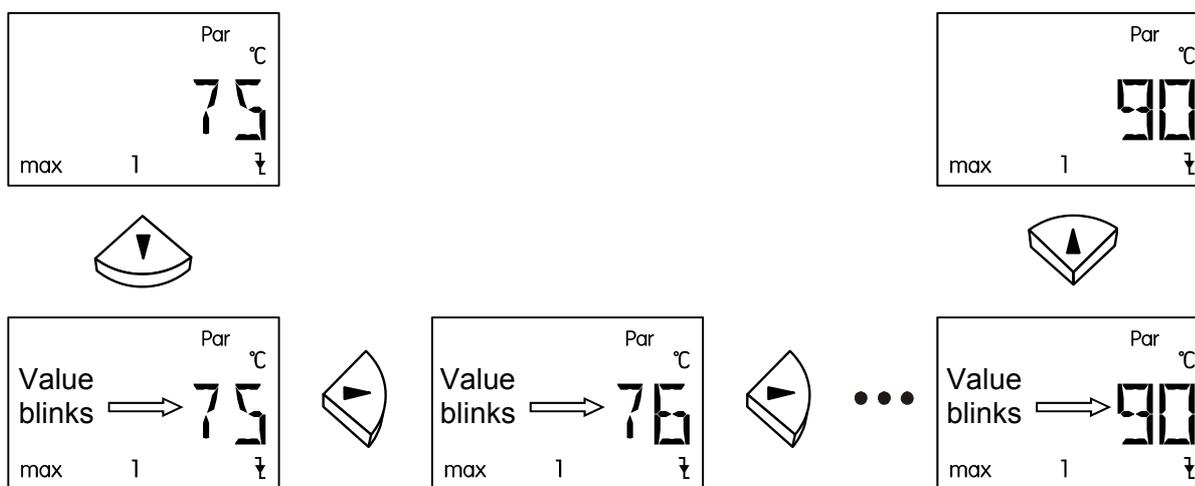
If a value is to be changed, press the arrow key. This value will then blink and can be set to the desired value with the navigation keys. Use the arrow key up to save the value.
