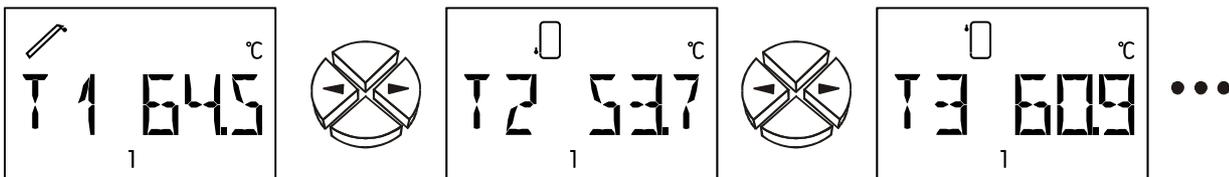
To the side of the display, the currently active outputs are identifiable on the green illuminated figures 1 - 3. If the speed control is active, the output 1 display flashes according to the speed stage.
