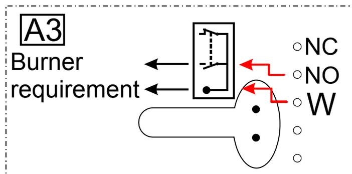
If the jumper is removed, then output 3 is potential-free.
