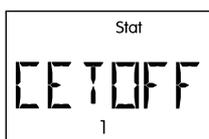
Collector - excess temperature - switch-off is active
