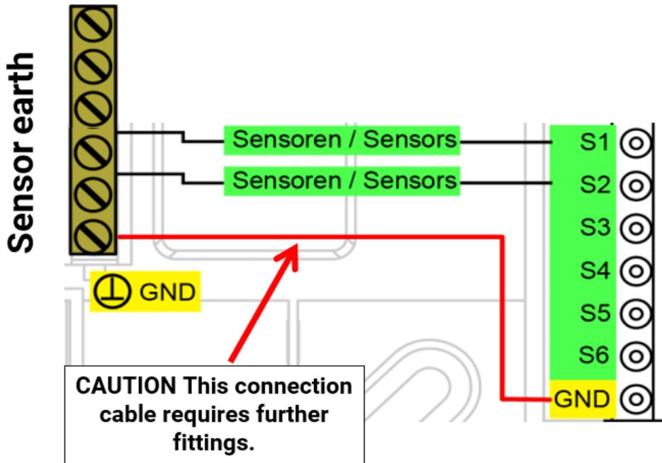
Sensors are always connected across the relevant sensor terminal (S1 – S6) and sensor earth (GND). There is an earth strip in the base. A connection to the GND terminal must be laid using this strip before the sensors are connected.
