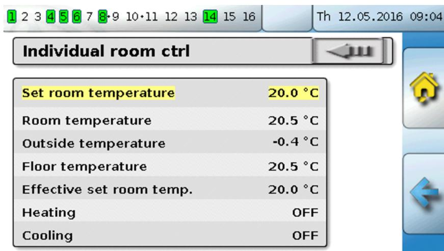
The screenshot shows a control interface for 'Individual room ctrl'. At the top, there is a navigation bar with numbers 1 through 16, where 14 is highlighted. To the right of the navigation bar, the date and time are displayed as 'Th 12.05.2016 09:04'. Below the navigation bar, the title 'Individual room ctrl' is shown with a back arrow icon. The main content area displays a table of room parameters:
