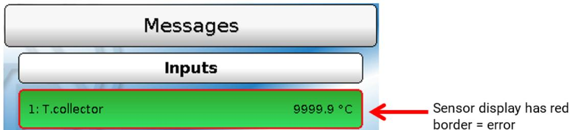
The display of 9999.9 °C for sensor 1 indicates an interruption (sensor faulty or lead break). If -9999.9 °C was displayed, it would mean a short circuit in the sensor or sensor lead.
