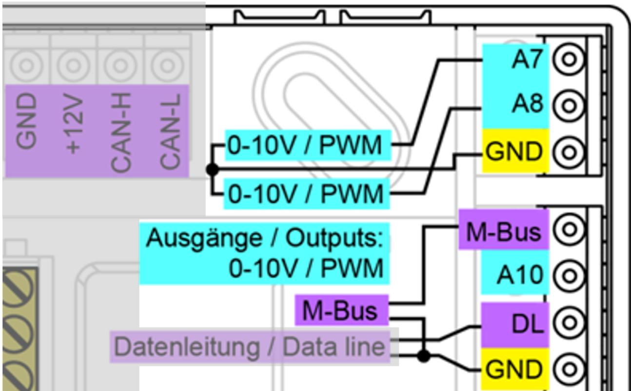
Outputs A7, A8 and A10 are the analogue outputs (0-10 V/PWM).
