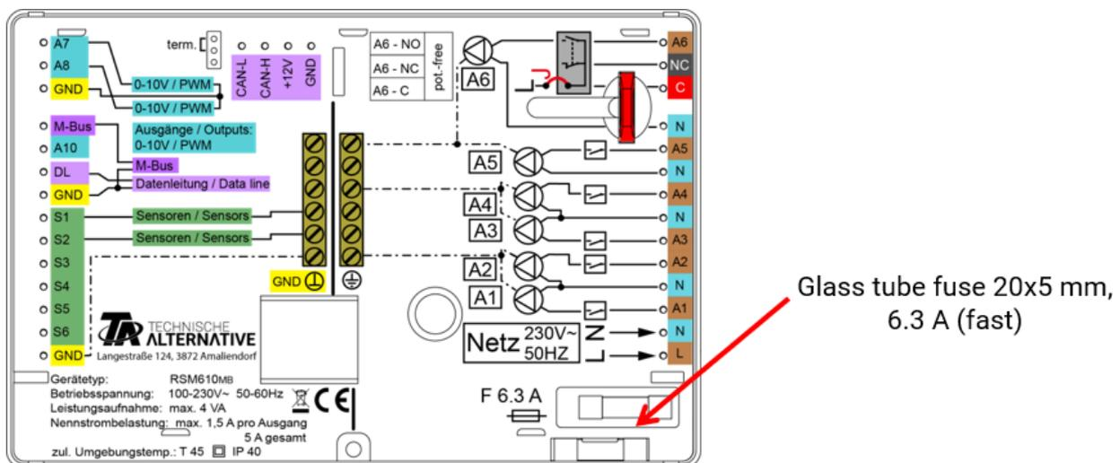
**Realistic temperatures but faulty operation of the outputs** indicates incorrect settings or termination. The device is in good order if it is possible to switch the outputs ON and OFF in manual mode; check all settings and termination.
