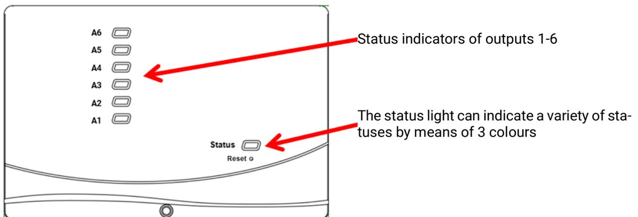
An active **Message** can be displayed by a change in a status indicator. This can be set in the **Parameters menu** of the **"Message"** function.
