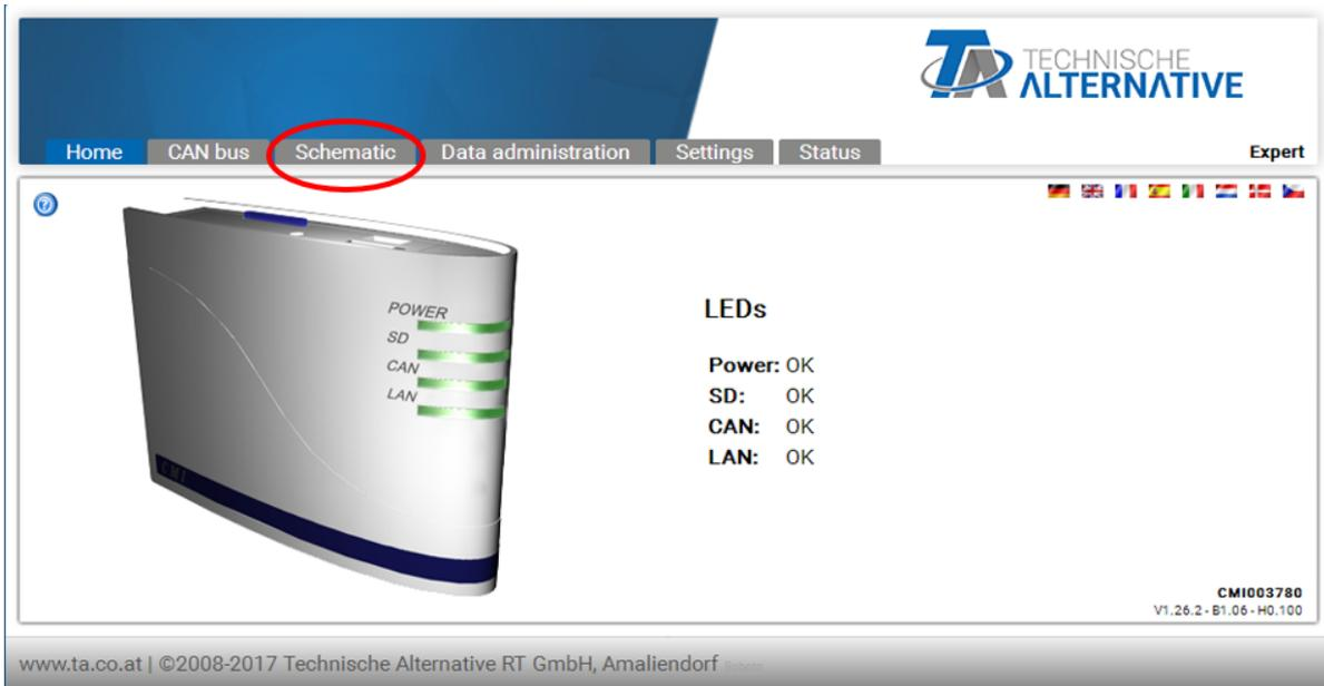
The operating status of the C.M.I. is shown with the LEDs. The current status of the LEDs is explained alongside.
