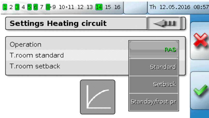
When you tap the required setting, it is changed and the required setting is displayed in the function overview.
