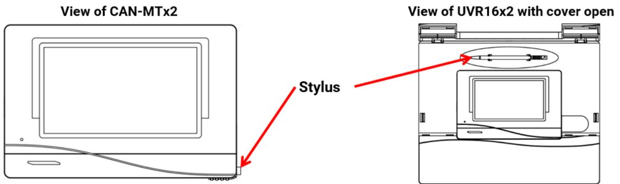
You can use the pen to tap operating fields on the screen and can scroll the view displayed by sliding it with the pen.
