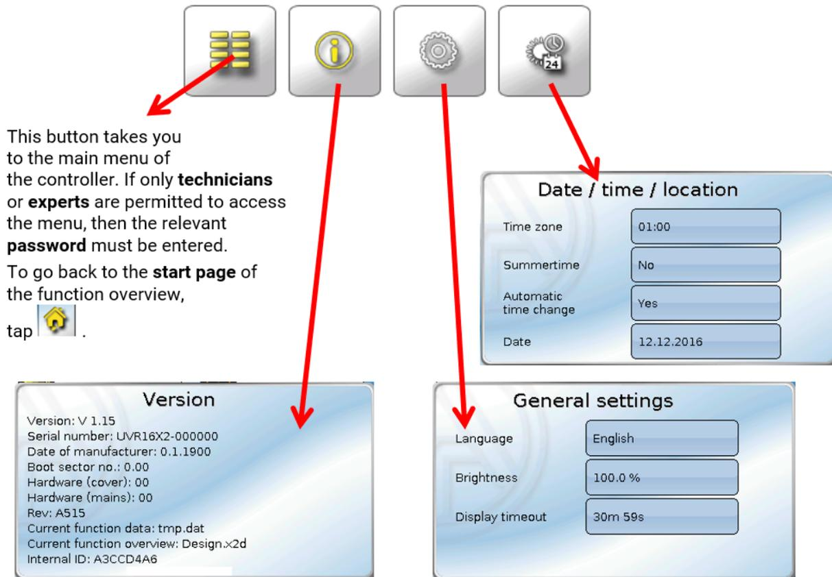
This button takes you to the main menu of the controller. If only **technicians** or **experts** are permitted to access the menu, then the relevant **password** must be entered. To go back to the **start page** of the function overview, tap
