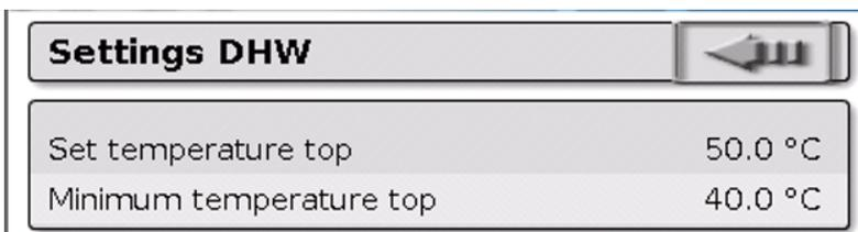
The DHW demand can be switched between two set temperatures via a time program from the **Time switch** function. The **Set temperature** applies inside the time window, and the **Minimum temperature** applies outside it.
