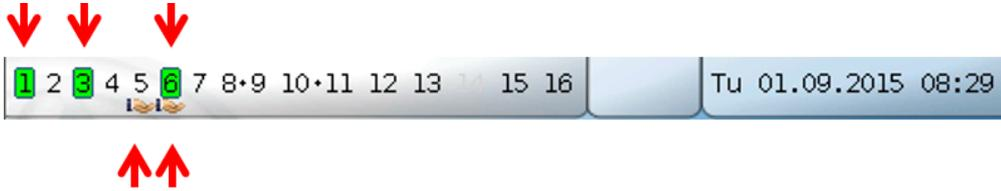
Output 5 has been **deactivated** manually (Manual/OFF) and output 6 has been **activated** manually (Manual/ON). Outputs that have been switched to Manual/OFF or Manual/ON are marked with a **hand symbol** under the output number.
