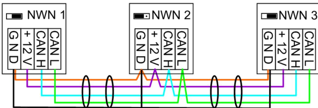
Each CAN network is to be provided with a 120 ohm BUS terminator at the first and last network subscriber (= **termination**). This is achieved with a plug-in jumper **at the back of the controller**. Each CAN network therefore always has two terminators (one at each end). Branch cables or a star topology are not permissible for CAN wiring.
