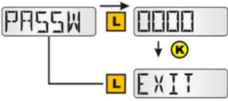
The purpose of this password is to block access to the CONFIG and VALUES menus. For access, enter the password set here. If **0000** is entered, no password is required. While the password is shown, long clicks can be used to go through the individual character places (active place flashes) and a short click increases a place by 1. A long click while the last place is active ends the entry process.
