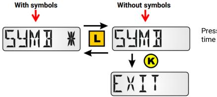
Press and hold the button for a long time to select the required display.
