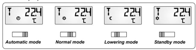
The signal reported at the controller corresponds to the room temperature changed using the rotary knob. The following signals are forwarded to the controller according to the switch setting:
