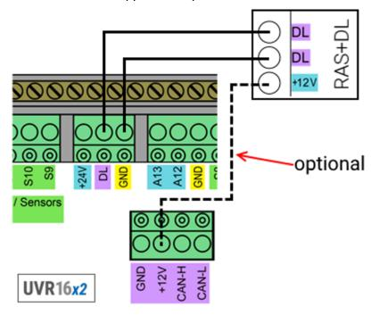
Any cable with a cross section of 0.75 mm<sup>2</sup> can be used for the data link (e.g. twin-strand) having a max. length of 30 m. For longer cables, we recommend the use of shielded cable.
