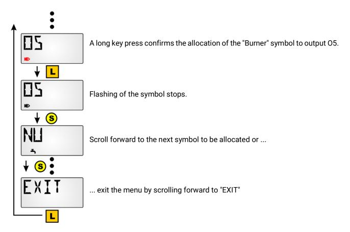
If the symbol is allocated to an **Output** or a **Digital CAN network input** (UVR1611), then it is shown in each display view for as long as the output or the digital network input is set to "ON".
