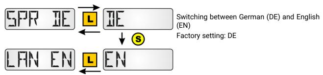
To activate the language selection the **RAS+DL** must be initialised by scrolling forward into the display level.
