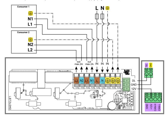
Mind the usage of suitable wire sizes and temperature resistance according to applicable norms.
