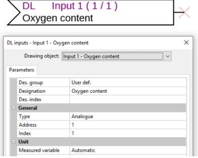
**Example:** Reading the oxygen content of a Lambda DL with address 1 via its index 1.
