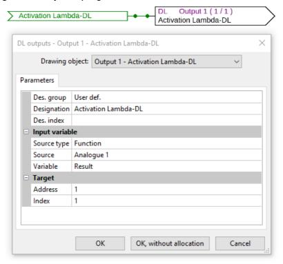
**Example:** Activation of a Lambda DL with DL address 1 via index 1.
