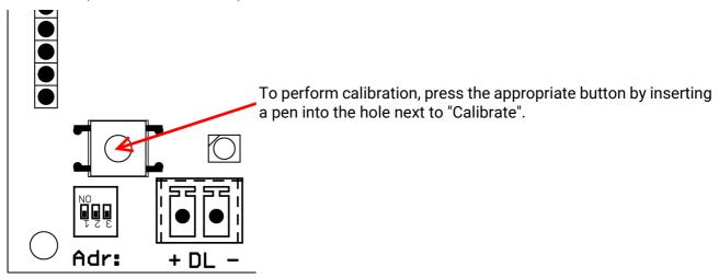
Throughout the entire calibration process, **4** is shown at index 5 (status) via the DL bus. In addition, index 1 displays the progress of the calibration process from 0 to 100 %.
