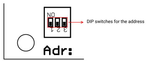
The new address is derived from address 1 (= factory setting) plus the sum of all the values cut.
