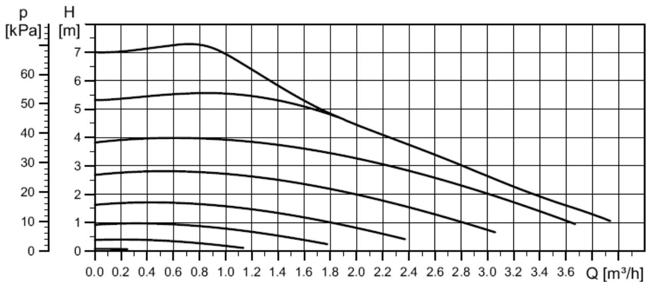
The pump operates in heating mode, meaning that at a 5 % PWM value, the pump will run at full speed. A break in the PWM lead therefore results in full pump speed.
