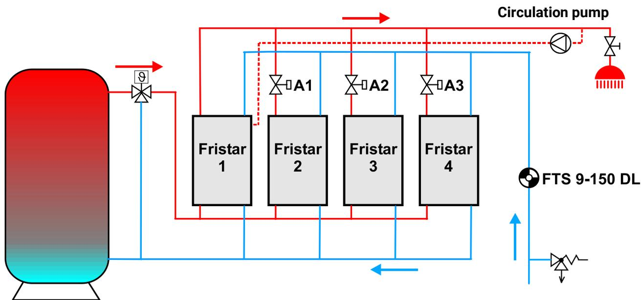
The circulation pump is connected only to the always ready **FRISTAR 2**.
