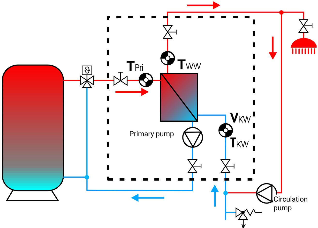
When the DHW circulation pump is switched on, the sensor ( $V_{KW}$ ) measures the flow rate and the primary pump is enabled.
