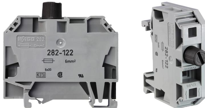
The SKL5x20 fuse terminal (including 6.3 A fast acting fuse) is used for external protection of the UVR610 controller. The internal fuse of the UVR610 can only be replaced at the manufacturer's factory. By connecting the fuse terminal to **L1**, the internal fuse of the device is bypassed. The fuse in the fuse terminal can be easily replaced on site.
