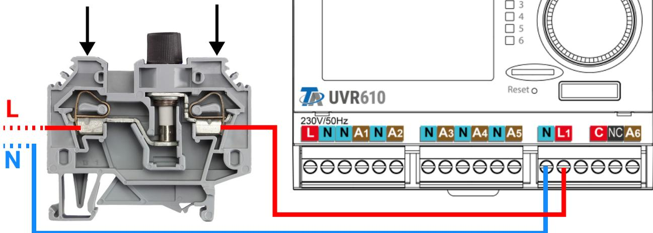
The fuse terminal is connected to **L1**. The direction as shown in the connection diagram must be observed (see "INPUT" printed on the top).
