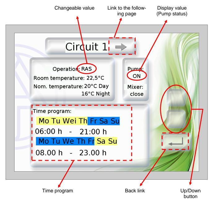
Programming of the **Time program** must be carried out so that the background for "**Normal**" and "**Selected**" are chosen in different colours. This makes it apparent which day is selected and therefore assigned ("Normal" = assigned, "Selected" = **not** assigned).
