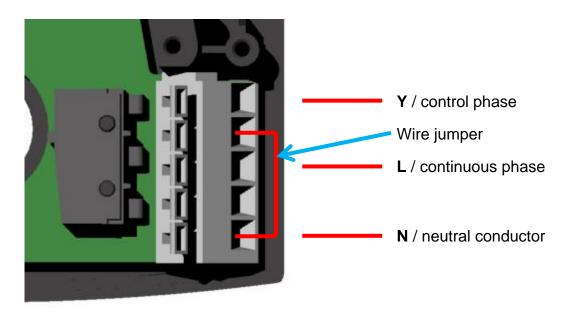
An **external voltage** may also be used for switching, if it cannot be ensured that the **Y** control phase has the same phase angle (L1, L2, L3) as the continuous phase or originates from the same electrical circuit:
