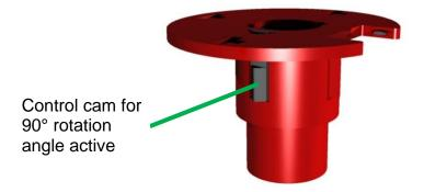
If the control cam has been broken out, but is no longer required, then it can be twisted by 180° and inserted into the groove, so that it can no longer actuate the limit switch:
