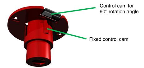
If a switching angle of 90° is required, then a second control cam must be inserted into the shaft. To do this, break the control cam (coloured grey in the drawings) out of the disc and slide it into the groove provided for this purpose.
