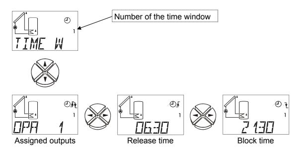
In the example, output 1 has been assigned to time window 1 (index). This output can be switched between 06:30 AM and 09:30 PM.
