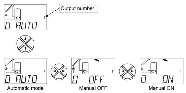
**IMPORTANT:** If the output is switched manually to ON or OFF this program diagram or these functions (e.g. anti-freeze, start function etc.) no longer have any effect on the output.
