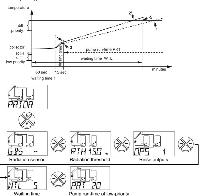
Radiation sensor **GBS 01** - non-standard accessory: Indicates a sensor input if a radiation sensor is used. If the radiation sensor exceeds the radiation threshold (RTH), the priority timer is launched.
