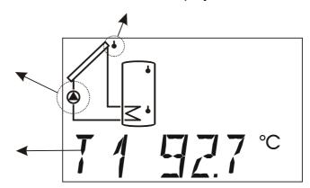
For programs, for which it is not possible to display a diagram in the display, the upper area remains empty. For some programs, the display was only approximately matched to the actual diagram, individual symbols may be missing.
