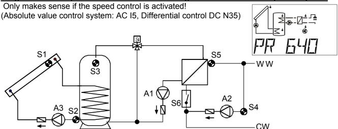
**WARNING:** Collector excess temperature limitation on output **A1** is activated ex works. This must be changed to **A3** or deactivated.
