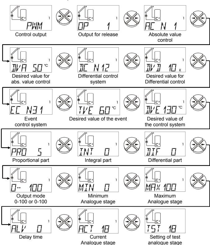
In this menu the parameters for the control output are specified.
