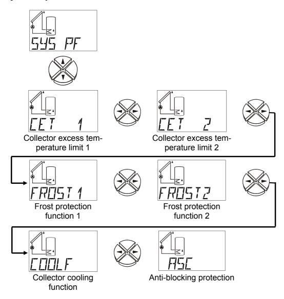
Two collector excess temperature limiter functions and two frost protection functions are available. These functions can be set completely independently of the program diagram selected.
