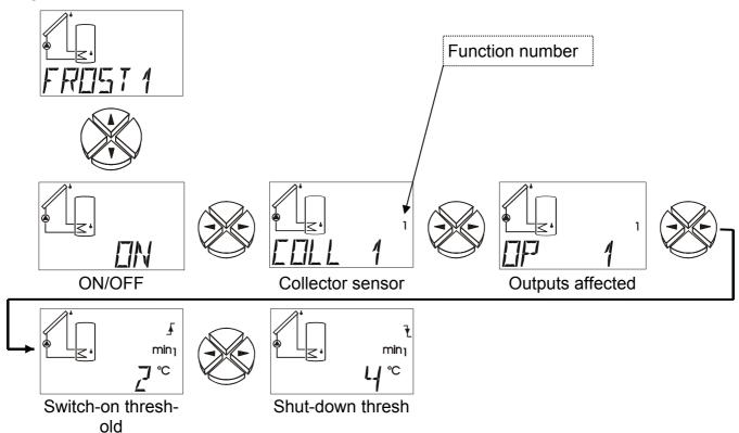
**ON / OFF** Frost-protection function ON/OFF (ex works<sub>1</sub> = ex works<sub>2</sub> = OFF)
