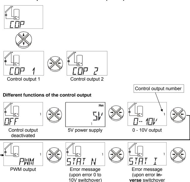
**OFF** Control output deactivated; output = 0V
