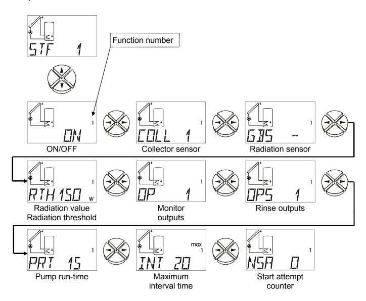
**ON / OFF** Start function ON/OFF (ex works<sub>1</sub> = ex works<sub>2</sub> = OFF)
