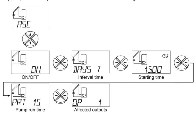
**ON / OFF** Anti blocking protection ON/OFF (ex works = OFF)
