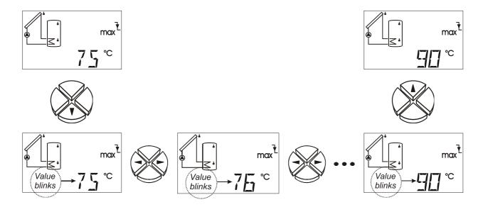
If a value is to be changed, press the arrow key. This value will then blink and can be set to the desired value with the navigation keys.
