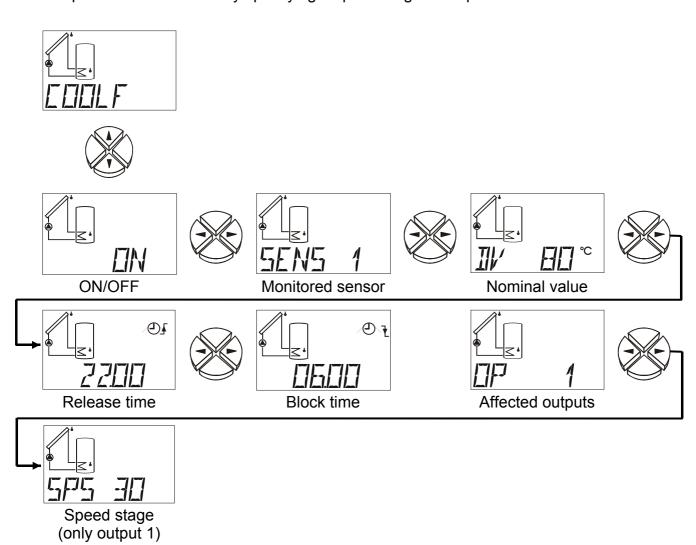
**ON / OFF** Collector cooling function ON /OFF (ex works = OFF)
