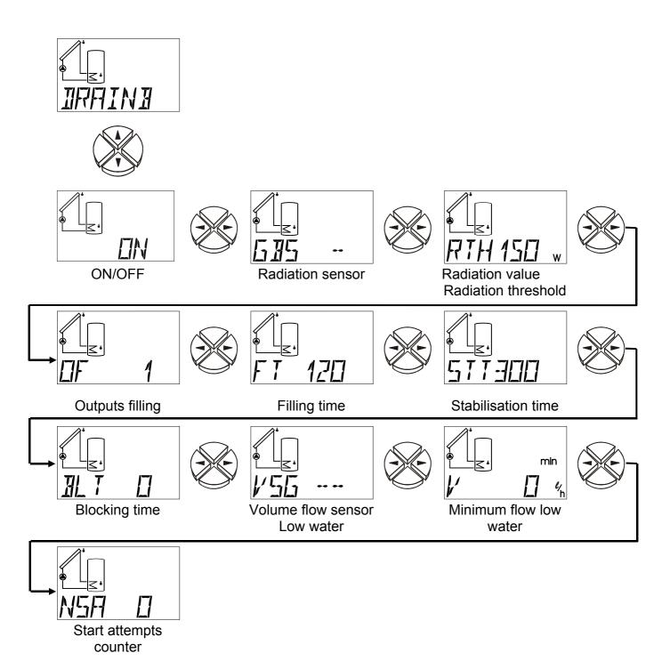
**ON / OFF** Drain-back function ON /OFF (ex works = OFF)
