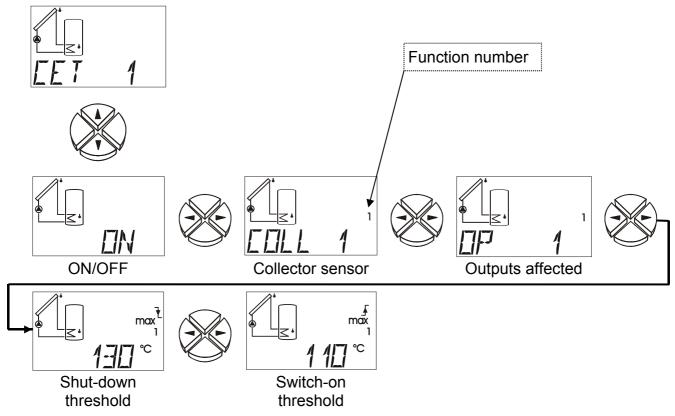
**ON / OFF** Collector excess temperature limit ON/OFF
