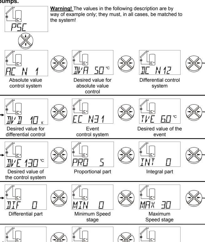
The behaviour of the control circuit is equal to that of the control outputs (COP); however, instead of 100 (COP) a maximum of 30 increments is available.
