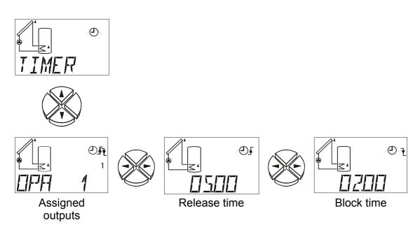
In the example the timer function is assigned to output 1. The output is released for 5 hours and blocked for 2.
