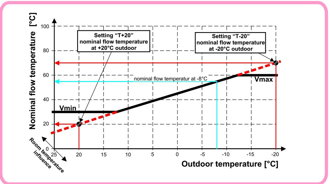
**Vmin, Vmax:** Minimal resp. maximal allowed flow temperature (limiting the heat curve)
