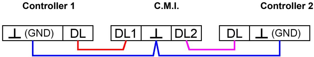
Any cable with a cross section of 0.75 mm<sup>2</sup> and a length of up to max. 30 m can be used for the data line (e.g. twin-strand). For longer cables, we recommend the use of shielded cable whereby the cable shielding must be connected with the sensor earth.
