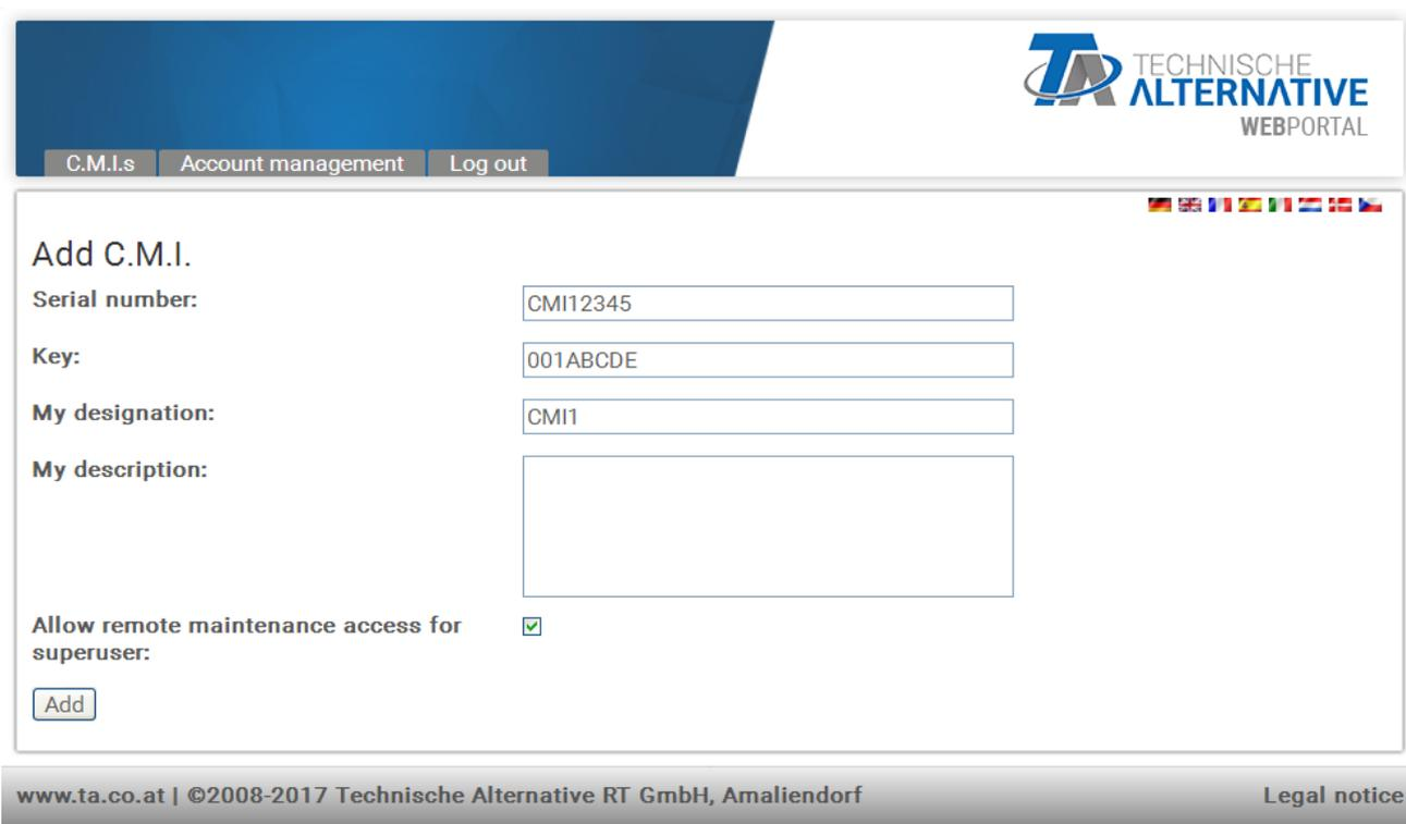
On the rear of the device is the **serial number** on the rating plate and the **key** on the key label. The key must be entered **without spaces**.
