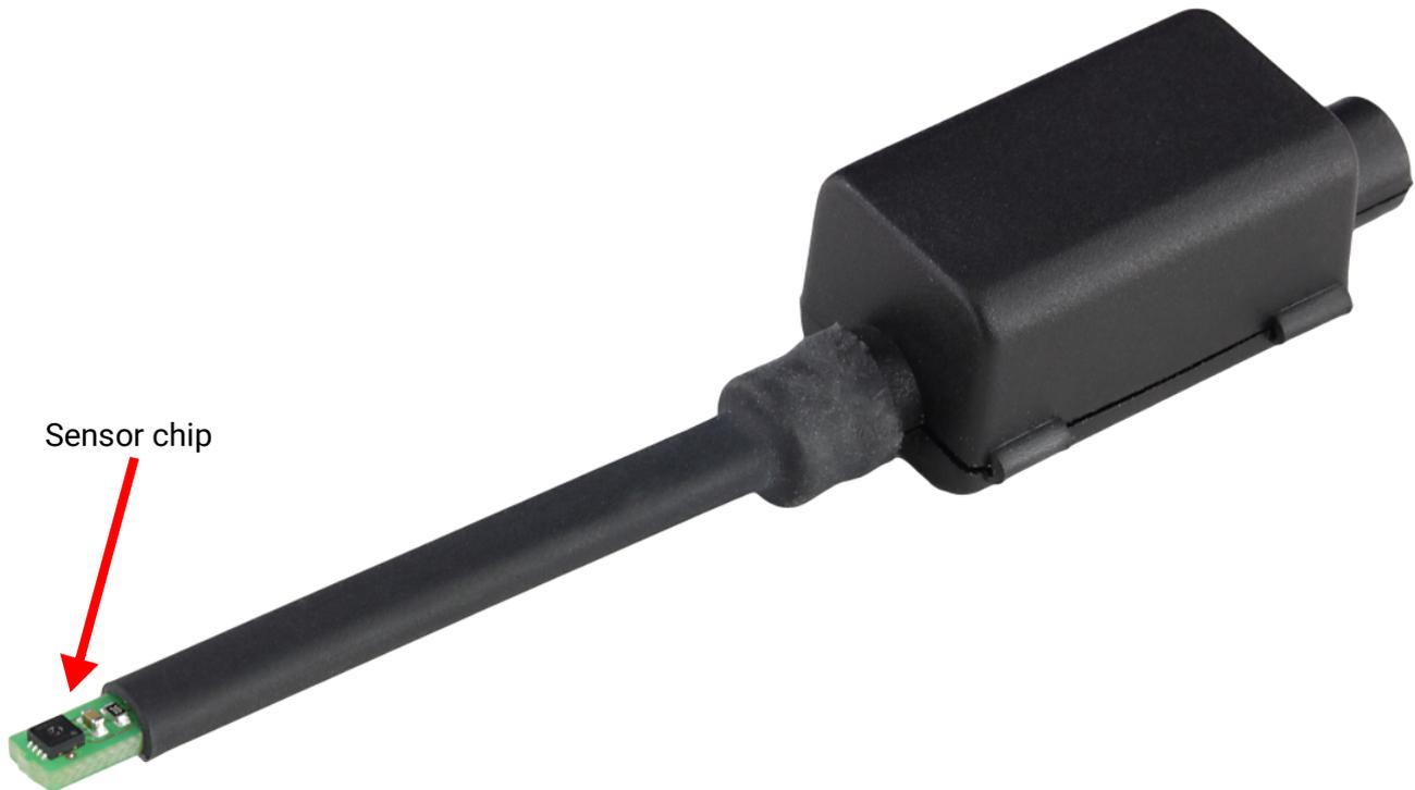
In the RFSE-DL, the humidity sensor is located on a 65 mm extension of the PCB which can be lengthened, for example, for mounting from the outside through a sauna ceiling.
