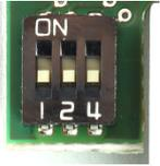
The **address** is set using the DIP switches. In the delivered condition, the address is set to 1 (factory setting).
