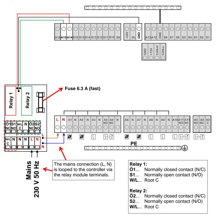
The relay module can be connected to any two outputs between A12 and A16 if these have been programmed as switching outputs.
