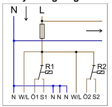
If the fuse is removed, both outputs will be potential-free whilst remaining connected to one another via root "W".
