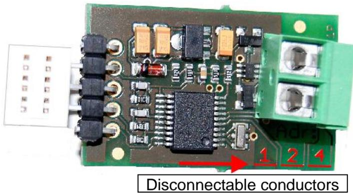
The **address** is specified on the adapter by breaking the conductors which are labelled 1, 2 and 4. These are located on the underside on the outer PCB edge. If none of the conductors are cut, the adapter is assigned address 1 (factory setting). Provided no other sensors are connected to the DL-bus, no change of address is required.
