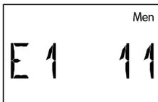
Here, the external sensor **E1** was allocated the sensor value of **address 1** with **index 1**.
