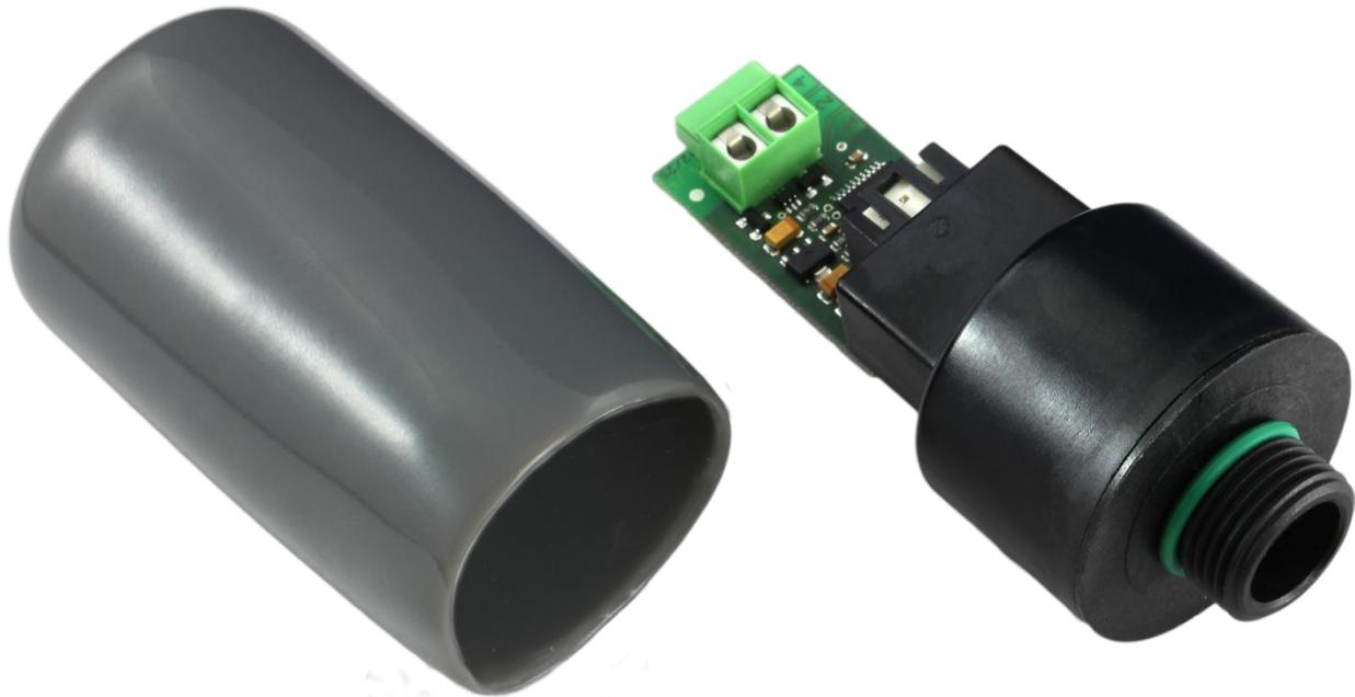
The pressure sensor PRS0-6DL is used to measure the physical variable, pressure. It is particularly suitable for determination of water pressure conditions in heating and service water circuits. The adapter electronics converts the measurement values into a serial digital signal suitable for the DL bus (data link).
