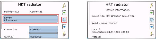
Device type contains either "HKT 12 V" or "HKT battery", depending on the type of power supply.
