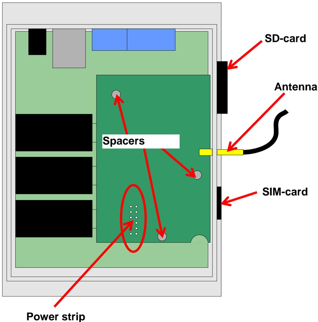
**Caution!** If the module is incorrectly put on the **power strip** (e.g. if the pins are left open), C.M.I. and also the GSM module can be **damaged**.
