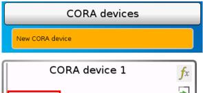
In the main menu, under "CORA devices", a New CORA device is selected. Once the device type has been selected, additional setting options appear.
