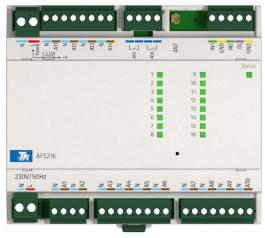
The **AFS216** actuating controller switches up to 14 thermal actuators. These 14 outputs for actuators are designed for continuous current up to 30 mA, individual pulses (start-up current) up to 0.5 A. In addition, 2 potential-free relay outputs are available under output 15 and 16. Finally, there are two further inputs for PT1000 temperature sensors.
