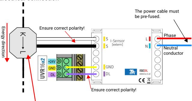
Each external current transformer is labelled with "K -> L" (or P1 -> P2), whereby the **electric current direction must be from** K to L (or P1 to P2) for positive metering.
