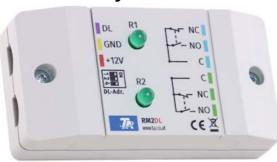
The **RM2-DL** switches 2 potential-free relays via DL bus. A 12 V supply (e.g. from the CAN bus) is also required. The relays have a maximum breaking capacity of 5 A.
