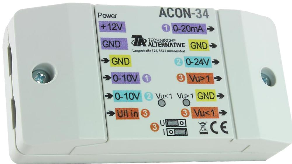
This device has been designed to adjust signals between UVR controllers and third party devices or industrial sensors.
