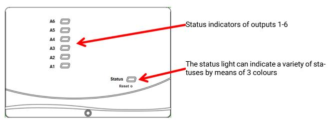
An active **Message** can be displayed by a change in a status indicator. This can be set in the **Parameters menu** of the "**Message**" function.
