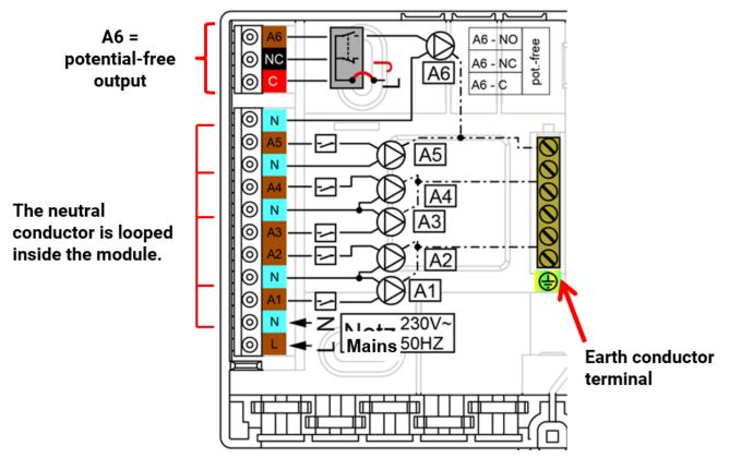
For maximum current load of the outputs, see the technical data.
