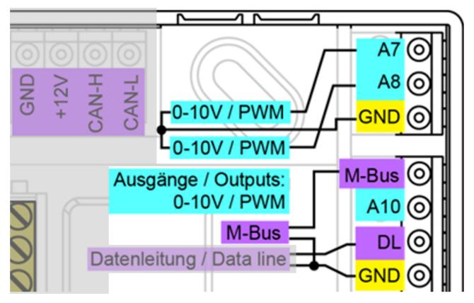
Outputs A7, A8 and A10 are the analogue outputs (0-10 V/PWM).
