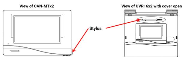
You can use the pen to tap operating fields on the screen and can scroll the view displayed by sliding it with the pen.
