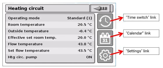
Operating mode shows the currently active operating mode. The operating mode is set by the controller setting for "Operation", the calendar function, the maintenance function, the "Window contact" status or the "External switch" status. Depending on the status of these functions and input variables, the operating mode may therefore vary from the internal setting for "Operation".
