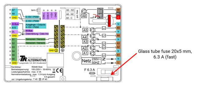
**Realistic temperatures but faulty operation of the outputs** indicates incorrect settings or termination. The device is in good order if it is possible to switch the outputs ON and OFF in manual mode; check all settings and termination.
