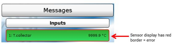
The display of 9999.9 °C for sensor 1 indicates an interruption (sensor faulty or lead break). If -9999.9 °C was displayed, it would mean a short circuit in the sensor or sensor lead.
