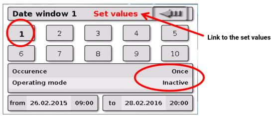
The calendar function is currently **Inactive**. Here you can define whether the calendar mode should be applied once or annually. Tapping the displayed **Operating mode** allows you to set the required operating mode:
