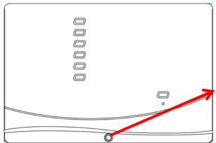
Unscrew the screws on the front and lift the cover.
