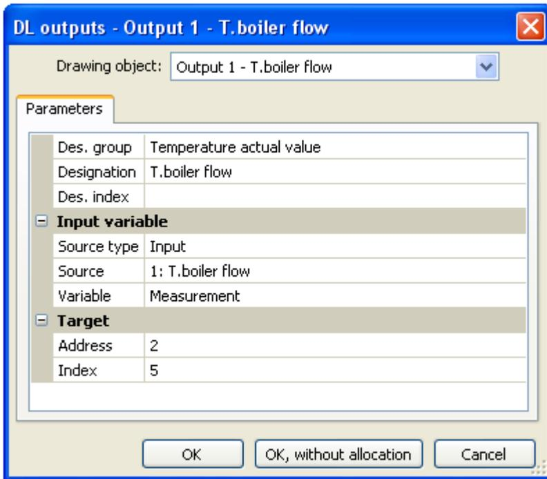
The input variable of the DL output must be an **analogue** numerical value.
