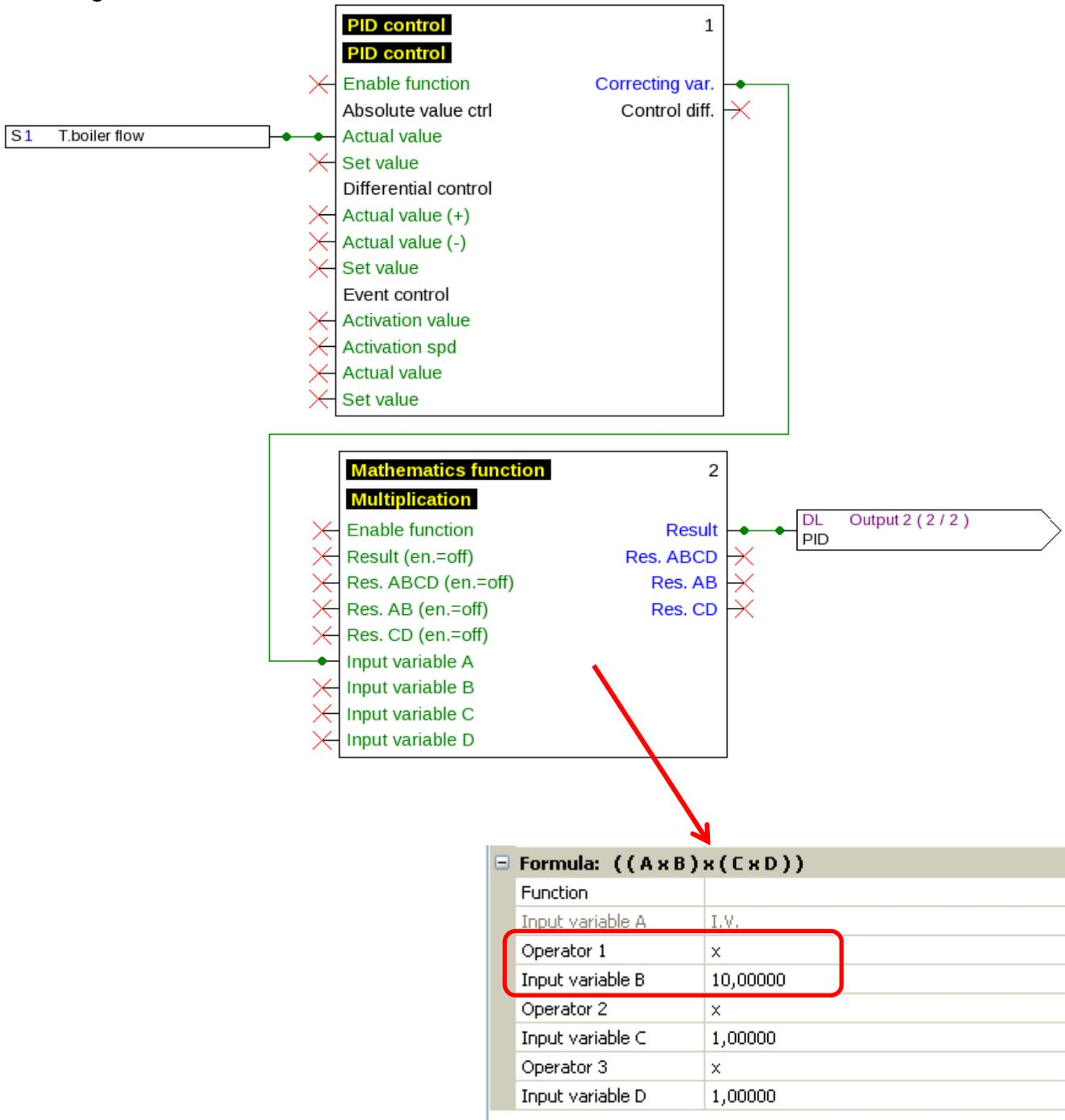
In the scaling function, a PID correcting variable of e.g. **60** results in **60.0 %**.
