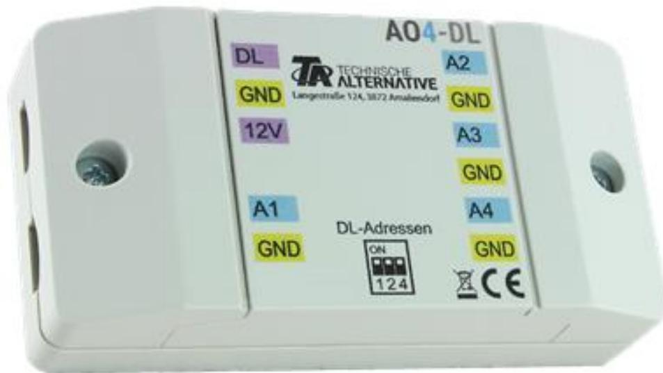
The **AO4-DL** module ("AO" = analogue output) enables an additional 4 analogue outputs for devices with X2 technology (e.g. UVR16x2, RSM610, CAN-I/O45).
