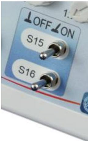
Using the two **changeover switches** for **inputs 15 and 16**, these inputs can be simulated as analogue temperature inputs or digital inputs, **depending on programming**.
