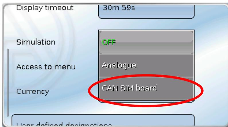
The simulated temperatures of **all** X2 devices are applied to a CAN network where the simulation is set to "**CAN SIM board**".
