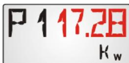
Current output of the heat quantity counter 1 in kW. For 4 figure numbers to be displayed, "P1" and "17,28" flash alternately.
