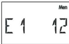
**Example:** The external sensor 1 has address 1, the measured room temperature is imported without offset values (index 2).
