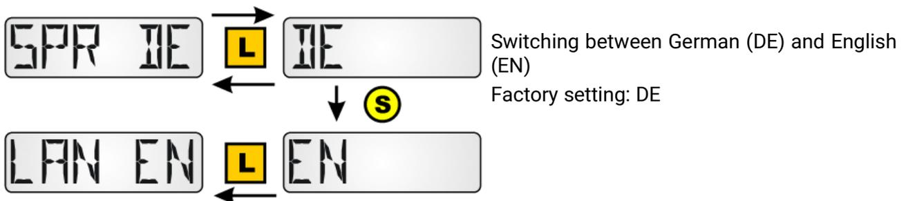
To activate the language selection the **RAS+DL** must be initialised by scrolling forward into the display level.
