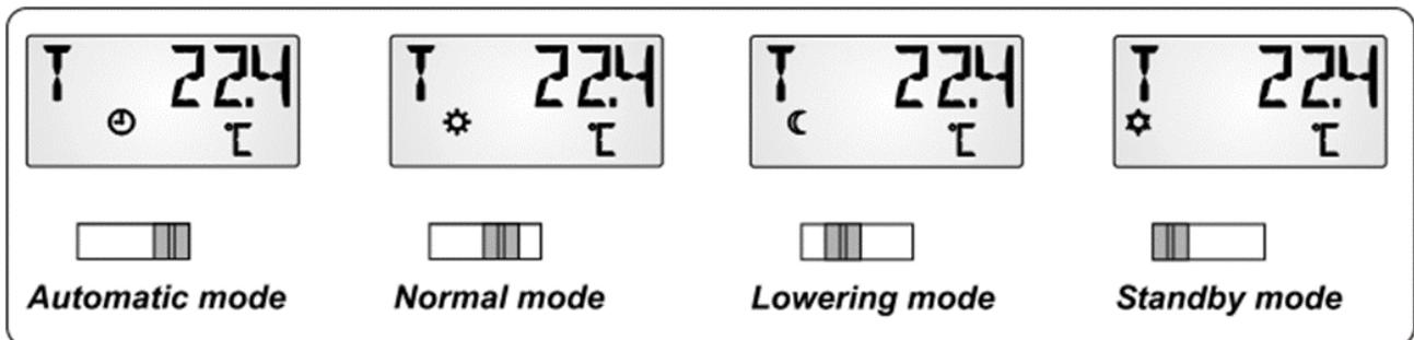
The signal reported at the controller corresponds to the room temperature changed using the rotary knob. The following signals are forwarded to the controller according to the switch setting:
