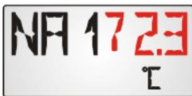
Current value of the analogue network input 1. For 3 figure numbers to be displayed, "NA1" flashes alternately with the value "72.3".
