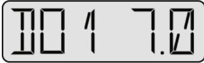
In this example, the RAS+DL is given a dimensionless value of **7.0** using a **DL output with index 1**.
