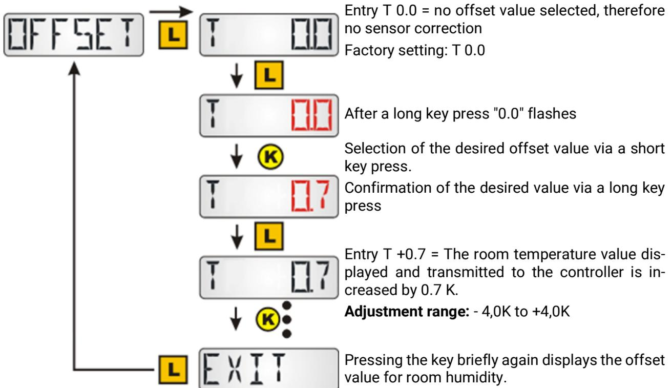
**Example:** If an offset value of 0.7K is set and a temperature of 21.0°C is measured, 21.7°C is indicated (index values 1 and 2). This corrected value is used in the sequence for all calculations and forwarded to the controller.
