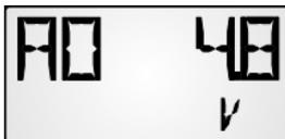
For controllers UVR61-3, UVR63, UVR63-H and ESR31 after display of the speed stage, the value of control output 1 (ANL1) can be displayed.
