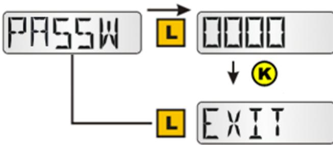
The purpose of this password is to block access to the CONFIG and VALUES menus. For access, enter the password set here. If **0000** is entered, no password is required. While the password is shown, long clicks can be used to go through the individual character places (active place flashes) and a short click increases a place by 1. A long click while the last place is active ends the entry process.
