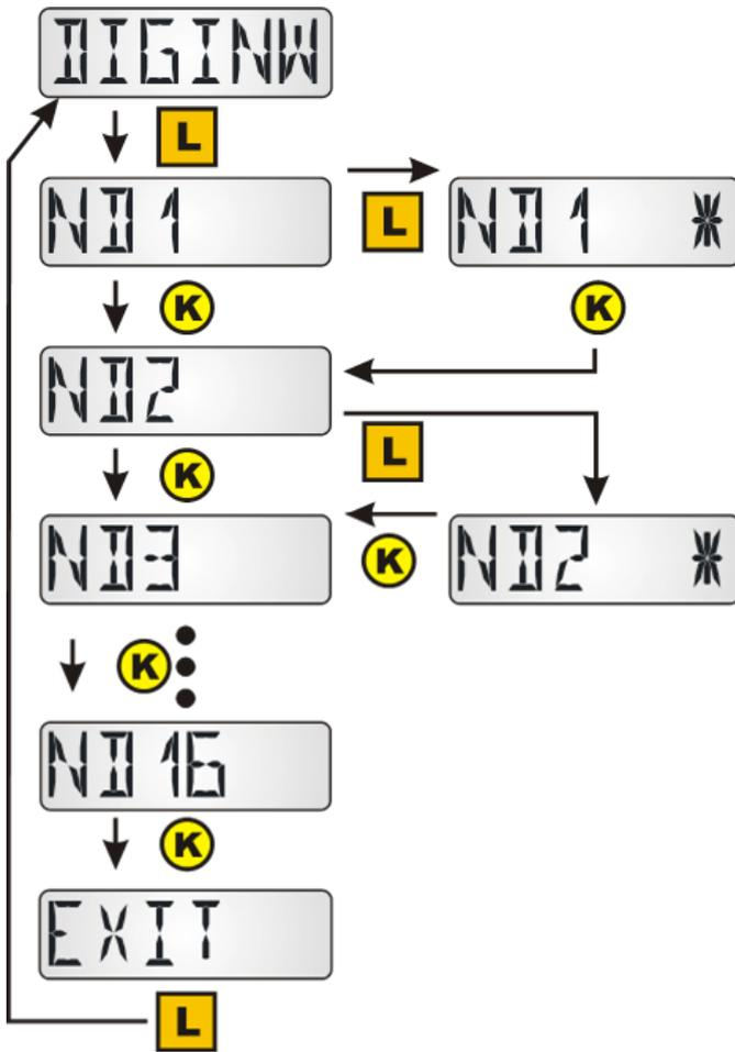
Selection via a long key press at the relevant digital network input. The selection is indicated by a star.
