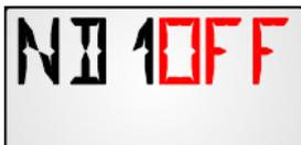
Current value of the digital network input 1. "ND1" and "OFF" flash alternately.
