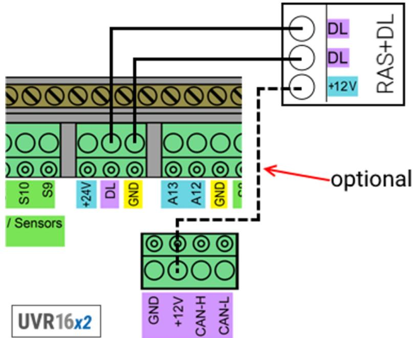
Any cable with a cross section of 0.75 mm<sup>2</sup> can be used for the data link (e.g. twin-strand) having a max. length of 30 m. For longer cables, we recommend the use of shielded cable.
