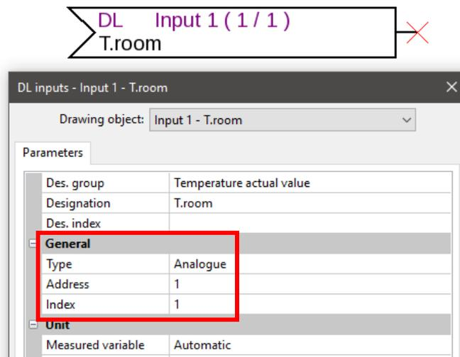
If the **measured variable** is set to "**Automatic**", no further settings are required here.
