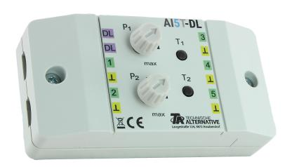
Mode of operation Programming The AI5T-DL (= "Analogue Input", button) translates signals for the data link (DL bus). These can originate from the two potentiometers, the 2 buttons (pulse/flip-flop in each case) or from up to 5 different external 0-10 V sources. It is recommended, that the 0-10V sensors that are being read out be connected to the same controller as the AI5T-DL itself.
