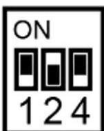
Position of DIP switches as per the example.
