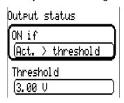
Depending on the technical attributes of the pump being controlled, it may thus be possible to set the output status to be ON only when the pump is actually running.
