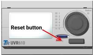
Pressing the reset button on the front of the controller briefly (with some narrow stick) and releasing it before the beep ends will restart the controller (= reset).
