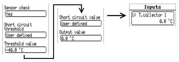
**Example:** Sensor 1 has fallen below -40 °C, so 0 °C is issued as the measurement, and a sensor error is displayed at the same time.
