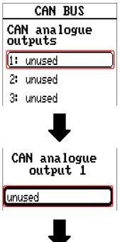
Specify the source in the controller which supplies the value for the CAN output.
