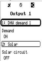
In this example, output 1 is controlled by two functions, and it has just been switched on by function 1 (DHW demand 1).
