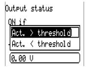
For the output status you can define whether the ON status should be issued above or below an adjustable threshold.
