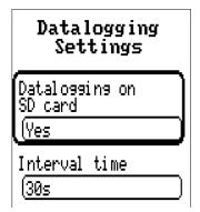
Here, you can define whether the logging values are stored on the SD card for the controller and if so, at what intervals.
