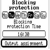
The outputs selected in the Output assignment will be switched on for 30 seconds on Tuesday and Friday at 4:30 p.m. if the output has not been active since the last controller start or since blocking protection was last initiated.
