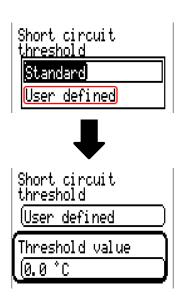
This setting is only displayed if sensor check is active and "Measured variable" is set to "User".
