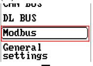
The UVR610-MODB controller can be used as master or slave for Modbus RTU485. In this menu, the Modbus settings are made and the inputs/outputs are programmed.
