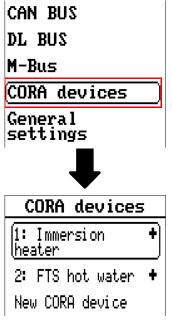
This menu allows CORA devices to be set and programmed wirelessly, and transmitted values to be imported.
