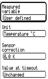
Every M-Bus input is assigned a **unit**, which can differ from the unit used by the M-Bus device. A wide range of units is available to choose from.
