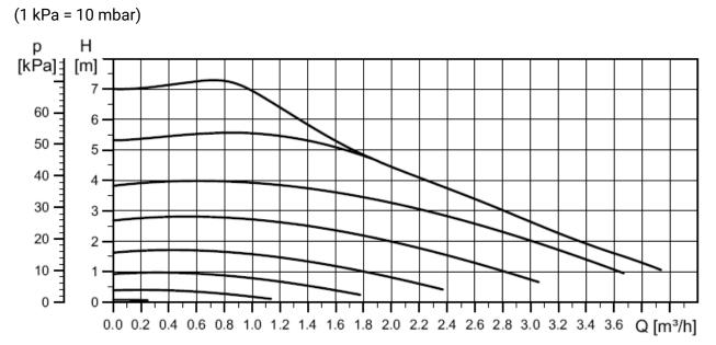
The pump operates in heating mode, meaning that at a 5 % PWM value, the pump will run at full speed. A break in the PWM lead therefore results in full pump speed.
