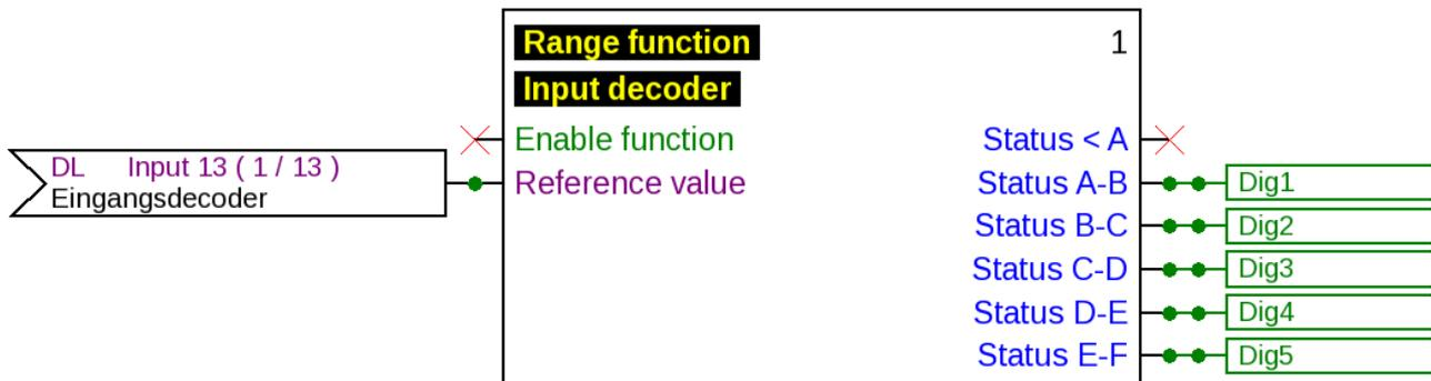
The DL input with **Index 11** outputs a number between 0 and 31, which is decoded by the binary decoder to produce a binary number with the input statuses. That DL input must therefore be linked to the input variable **Reference value** (as shown in the graphic).
