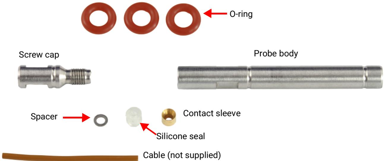
Guide the screw cap, spacer, silicone seal and contact sleeve onto the cable. Strip about 5-10 mm of insulation from the cable.
