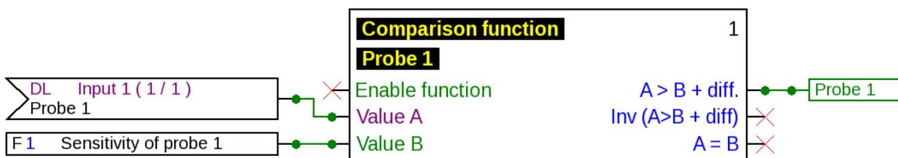
In the example, the first probe (**P1**) of an NME5-DL (address **1**) is compared with a fixed value. The comparison function does not output a digital value with **ON** until the value of the current flow exceeds the set fixed value **F1**.
