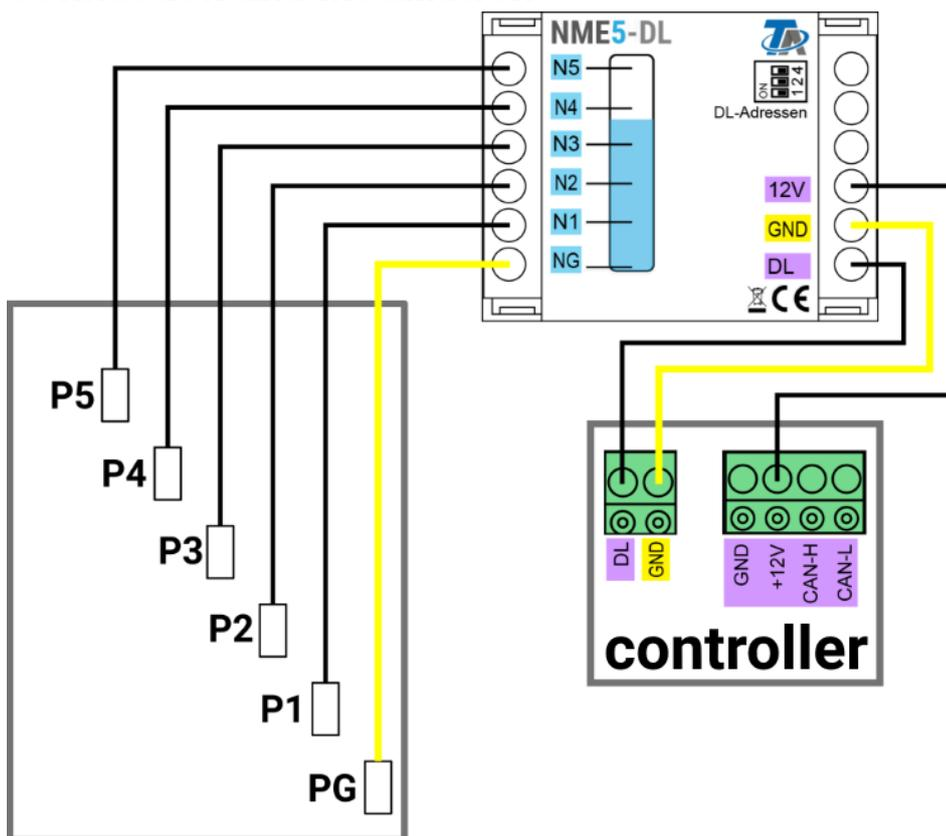
The probes are placed in the cylinder in ascending order, with the emitter (**PG**) in the lowest position. The probes must not touch each other in the cylinder. All probes are identical in construction – they only differ in connection and installation position.
