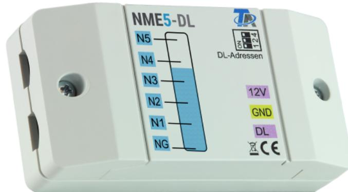
The **NME5-DL** level measuring unit measures how full cylinders, cisterns, etc. are using the current flow between an emitter (connection **PG**) and up to 5 probes (**P1-P5**). **The device is only compatible with controllers with x2 technology.**
