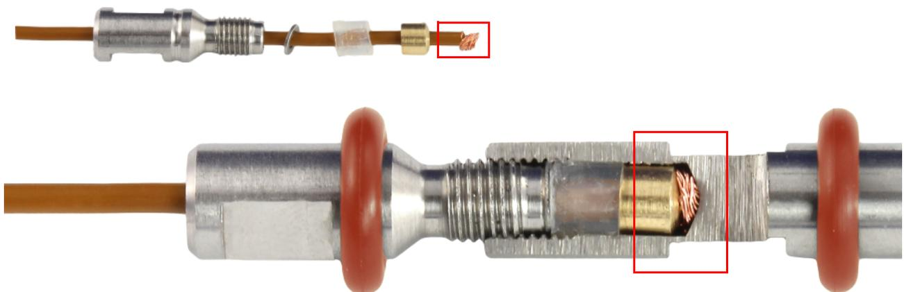
Finally, the screw cap is attached and the O-rings are placed on the notches. This process is the same for all probes (including the emitter PG).
