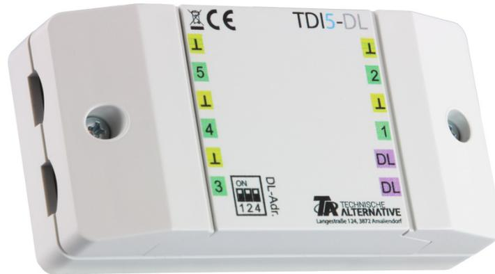
The TDI5-DL (Temperature and Digital Input) translates up to five signals for the data link (DL bus), which can be either a digital signal (On/Off) or the measurement from a PT1000 sensor. **Digital signals must be potential-free.**
