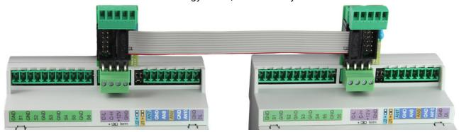
The ribbon cable does not fully comply with the specifications of the CAN bus protocol, but this is irrelevant given its short length (123 mm).
