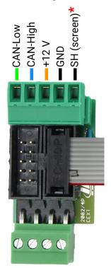
\*The 5th pole (on the right on the terminal) is for the screen of the CAN bus cable.
