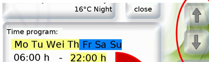
The background and/or the font colour of the switching time changes (dependent on the programming) and up/down arrows appear in the programmed area.
