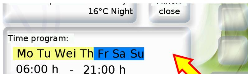
The arrows disappear if another area of the screen is touched. The changed switching time returns to the original background/font colour. The changed switching time is displayed.
