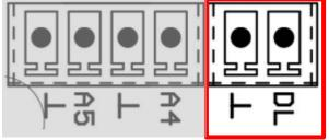
The DL bus consists of just 2 wires: **DL** and sensor earth ( $\perp$ ). The DL BUS itself supplies the necessary power for the DL BUS sensors.
