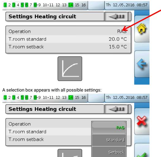
When you tap the required setting, it is changed and the required setting is displayed in the function overview.
