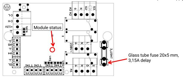
If the status LED indicators are switched off, this indicates failure of the power supply for the
