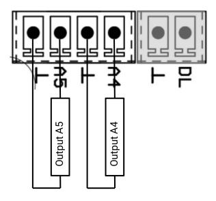
The connections A4 and A5 are the positive poles; the connections  $\perp$  are the negative poles. When programmed as a "switching output", a HIREL-230V or HIREL-PF auxiliary relay can be connected.
