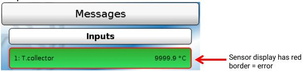
The display of 9999.9 °C for sensor 1 indicates an interruption (sensor faulty or lead break). If -9999.9 °C was displayed, it would mean a short circuit in the sensor or sensor lead.
