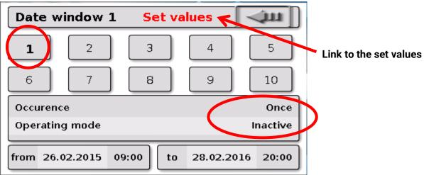
The calendar function is currently **Inactive**. Here you can define whether the calendar mode should be applied once or annually. Tapping the displayed **Operating mode** allows you to set the required operating mode:
