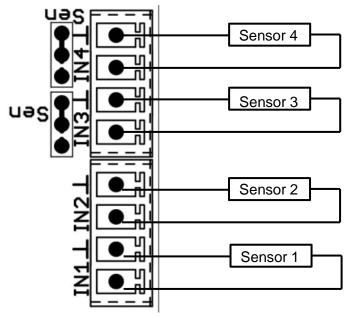
By repositioning the jumper, the inputs IN3 and IN4 can be switched to measuring voltage up to 10 V. However, sensor values can then no longer be recorded.
