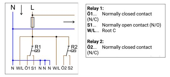
Both relay outputs are protected by the fuse on the relay module. Terminal "W" therefore corresponds to phase conductor "L".
