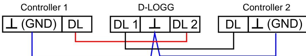
Any cable with a cross section of 0.75 mm<sup>2</sup> can be used for the data link (e.g. twin-strand) having a max. length of 30 m. For longer cables, we recommend the use of shielded cable. If the data from two controllers is to be acquired by the data converter, then separate shielded cables must be used to provide protection against crosstalk errors. The data conductors must never be in the same cable as the CAN bus.
